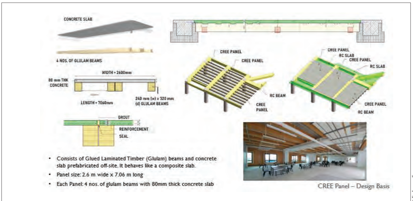
The prefabricated hybrid timber-concrete slab system (CREE) on the Eunoia Junior College project.
