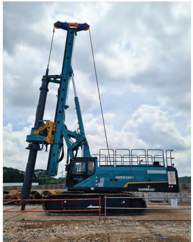
ALL IMAGES: The Sunward SWDM320HL low-mast rotary drilling rig is available in the Singapore market. The machine has a maximum drilling diameter of 2,500 mm and maximum drilling depth of 43 m.
