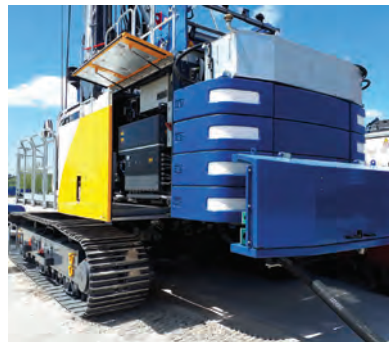
TOP: The new Bauer electric eBG 33 falls in the mid-range segment of the drilling rig series with a drive power of more than 400 kW.
