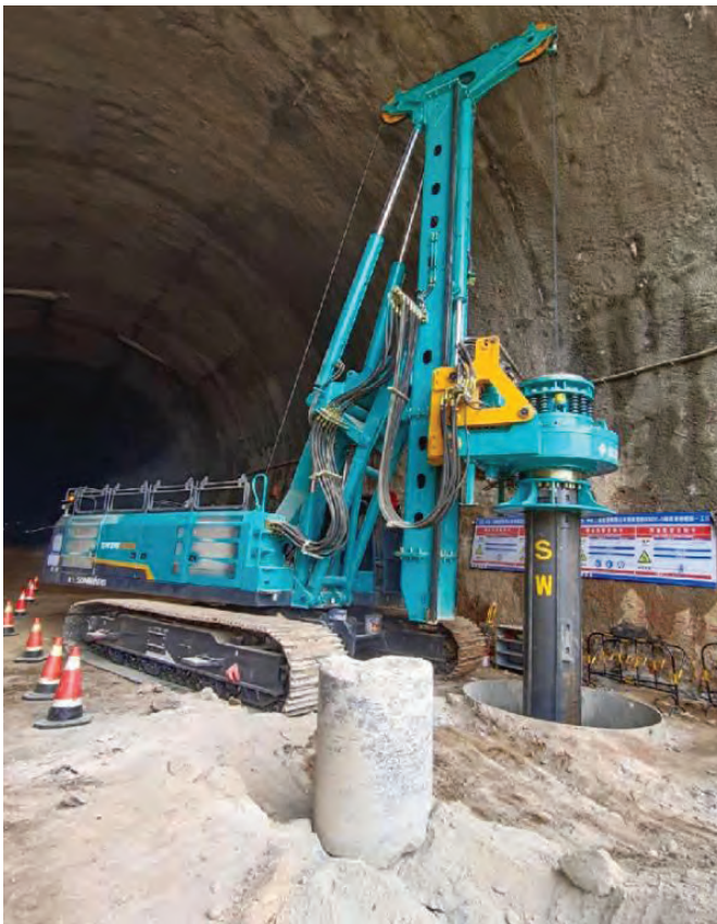
ALL IMAGES: The Sunward SWDM320HL low-mast rotary drilling rig is available in the Singapore market. The machine has a maximum drilling diameter of 2,500 mm and maximum drilling depth of 43 m.
