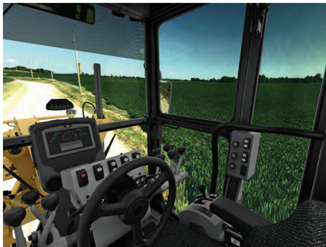
ABOVE AND LEFT: With 45 years of refinement, the 140 GC's conventional steering wheel and lever controls are familiar to operators and ensure positive control.
