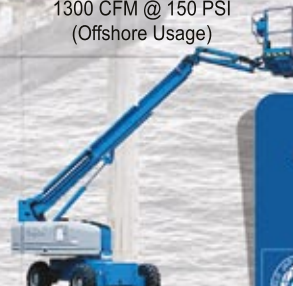
Boom Lift Working Height (6 - 41 Metres)
