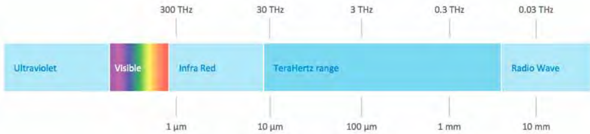
ThruVision operating frequency of 0.25 THz versus millimetre wave (~100GHz) scanners (as shown on the electromagnetic spectrum)
