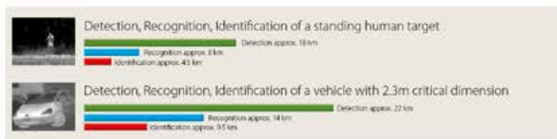
Actual range may vary depending on camera set-up, environmental conditions, user experience and type of monitor or display used. Assumptions: 50% probability of achieving objective at specified distance given approximately 2°C temperature difference and 0.82 / km atmospheric attenuation factor. DR according to MIL-STD-181C.
