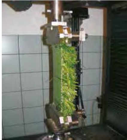
Resistance tests on the joints in synthetic grass surfaces carried out using the direct stress method, according to EN 12228 European Standards.
