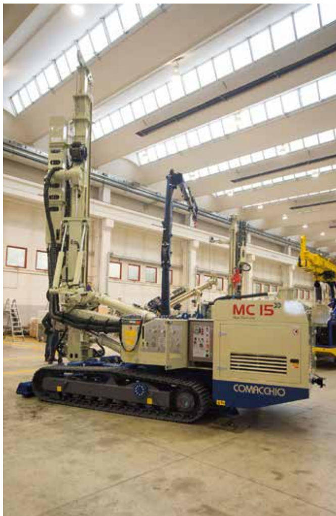
Left and right: The new Comacchio MC 15 hydraulic drilling rig is suitable for various ground engineering works, from micropiles to jet grouting, as well as anchor drilling. Here some MC 15 machines being shown during the company's open house at its Riese Pio X facility in October 2013. Foundation Associates Engineering Pte Ltd is the Singapore agent for the full range of Comacchio hydraulic rigs.
