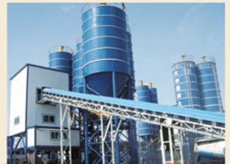
Ready- mixed Concrete Batching and Mixing Plant
