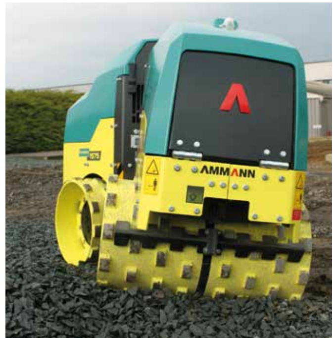
Rammax 1575 CI with articulated pendulum steering for excellent traction and powerful compaction.
