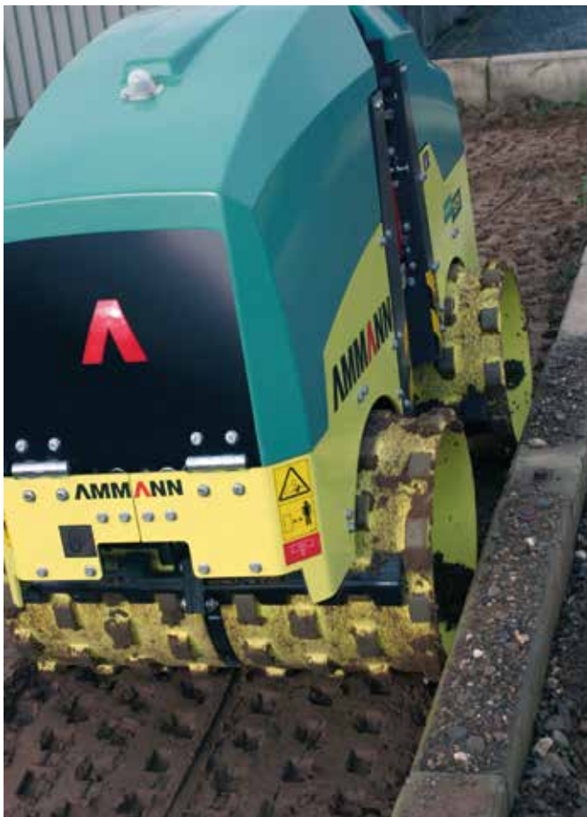
The Rammax 1575 CI trench roller enables sensitive steering by remote control, even alongside kerbstones.
