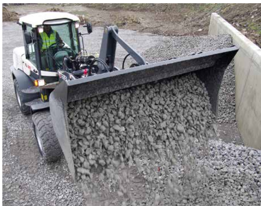
Top and above: Terex's TL120 wheel loader comes with far more than just a more powerful EU Stage IIIB engine; it has a new Terex Smart Control operating system, a quieter cab offering a better view for the operator and a new intuitive cooling system.
