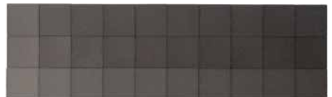
Saturation series for black iron oxide pigments iron oxide 1, iron oxide 2 and Bayferrox TP LXS 5253 (from bottom to top) with 1-percent graduation from left (1 percent) to right (10 percent). The blocks were made with white cement.
