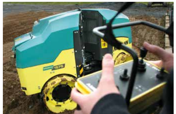
Infrared and cable remote control are standard features on the Rammax 1575 CI.
