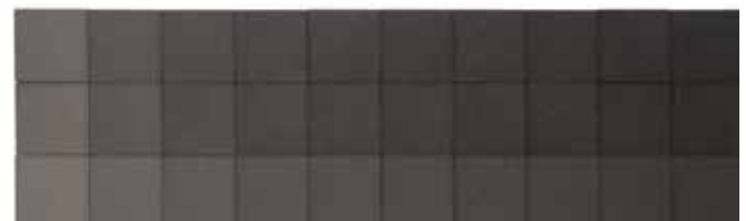
Saturation series for granular black iron oxide pigments (from bottom to top) iron oxide 3, iron oxide 4, Bayferrox TP LXS 5255 in 1-percent graduation from left (1 percent) to right (10 percent). The blocks were made with white cement.
