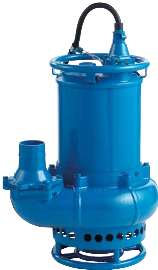
Left: The GPN415 features a motor output of 15 kW, maximum capacity of 4.1 cu m/min, discharge bore of 100 mm and maximum head of 21.6 m.
