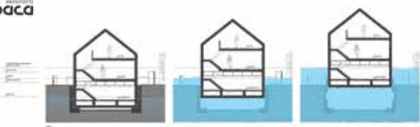
Indicative diagram of the showing the movement of the building in medium and high flood events. Photo: © Baca Architects
