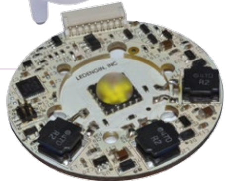
Light Sources LuxiTune dimmable and colour tunable LED light engine By LED Engin
