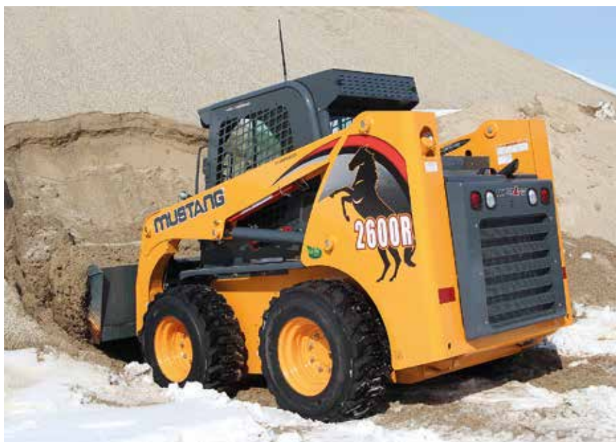
Top and above: The Mustang 2600R full-sized radial lift skid steer loader.
