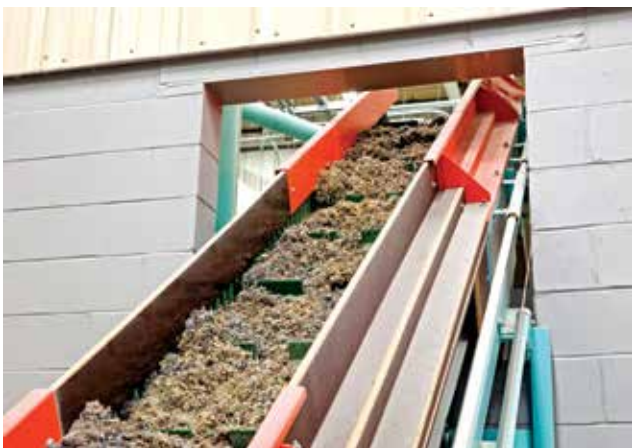
Interface recycles carpet tiles in a composite process that fully separates the backing, enabling yarn to be recycled into new yarn. Photo: © Interface
