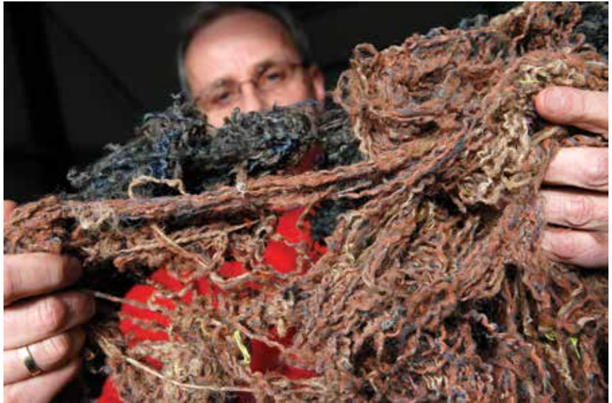
Interface recycles yarn to yarn and backing to backing, ensuring carpet tiles are part of a closed loop system where the separated nylon yarn feeds into new products. Photo: © Interface
