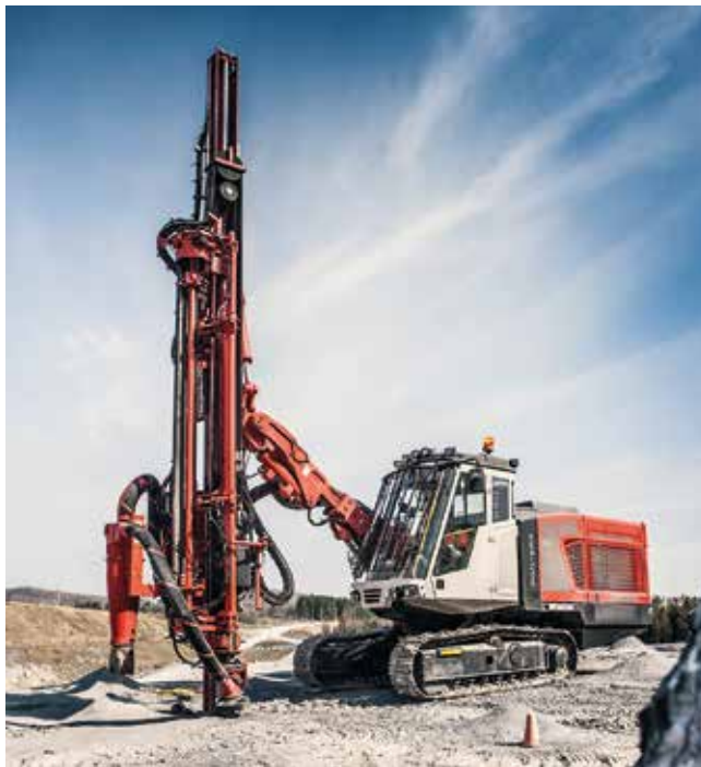
Left: The DP1500i is one of the two models in the new Pantera DPi 6.0 drill rig family. It is designed for hole sizes of 102 – 152 mm.
