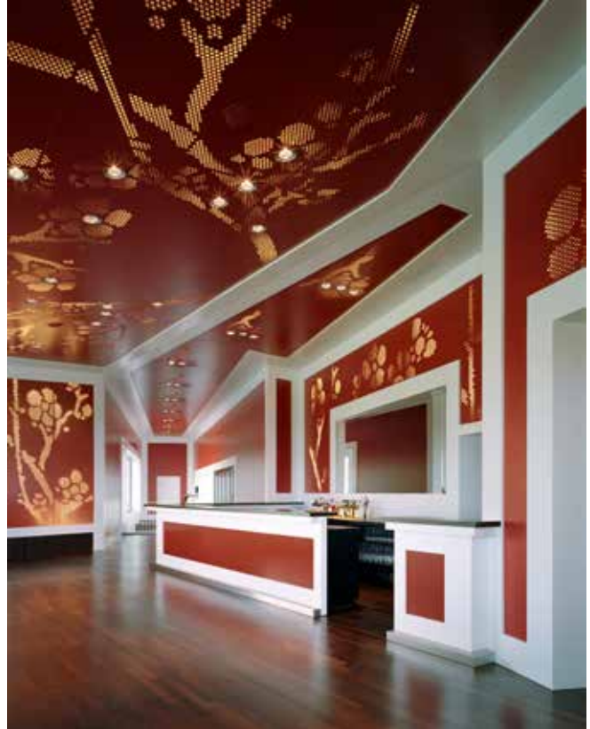
At the Golf Club Lake Sempach in Switzerland, the Topperfo Graphic System was specified for the walls and ceiling.
