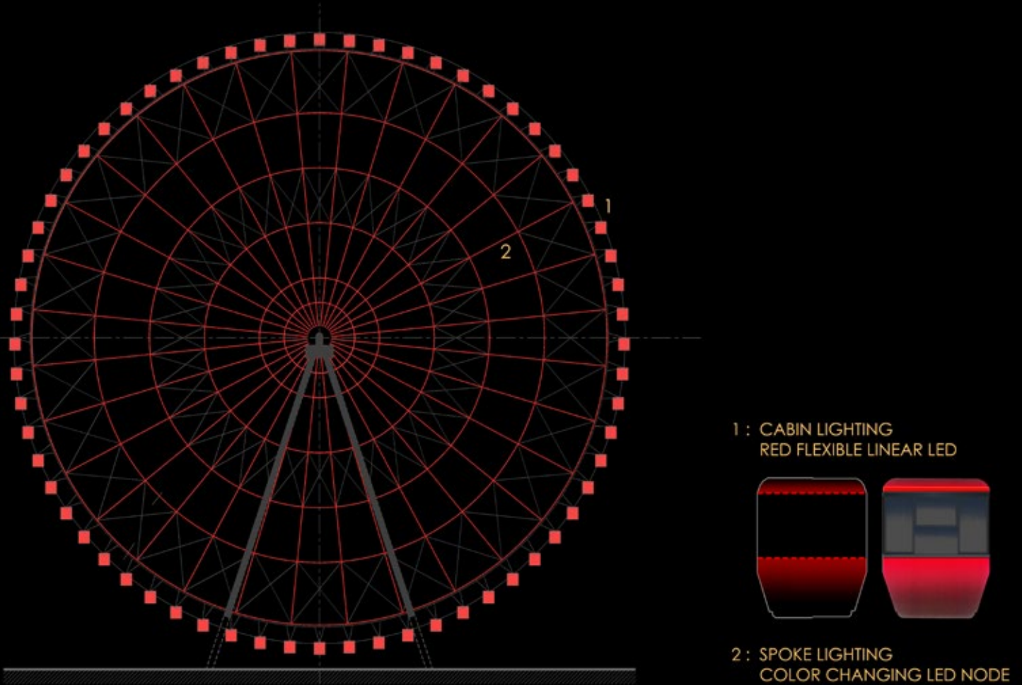
The position of lighting installed on the wheel
