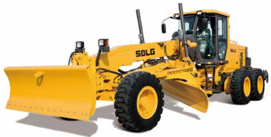
The G9190 motor grader was recently launched into the Indonesian market. Featuring an operating weight of 15.8 t and powered by a 148 kW Deutz engine, the machine can deliver traction force of up to 82 kN.
