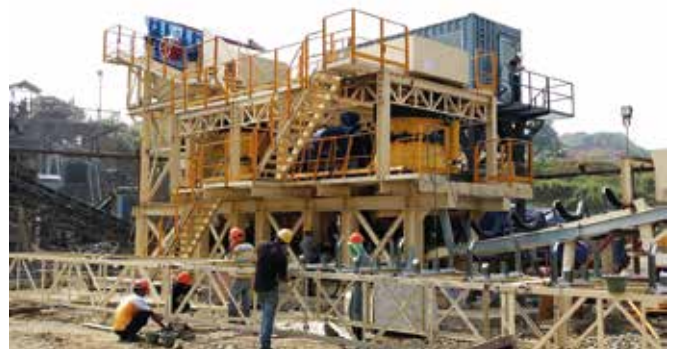
Trimax NS300 secondary cone crusher, Trimax NH400 tertiary cone crusher and Trimax ADplus (1,525 mm x 3,660 mm) x 2 deck vibrating screen on a skid-mounted prefabricated structure.
