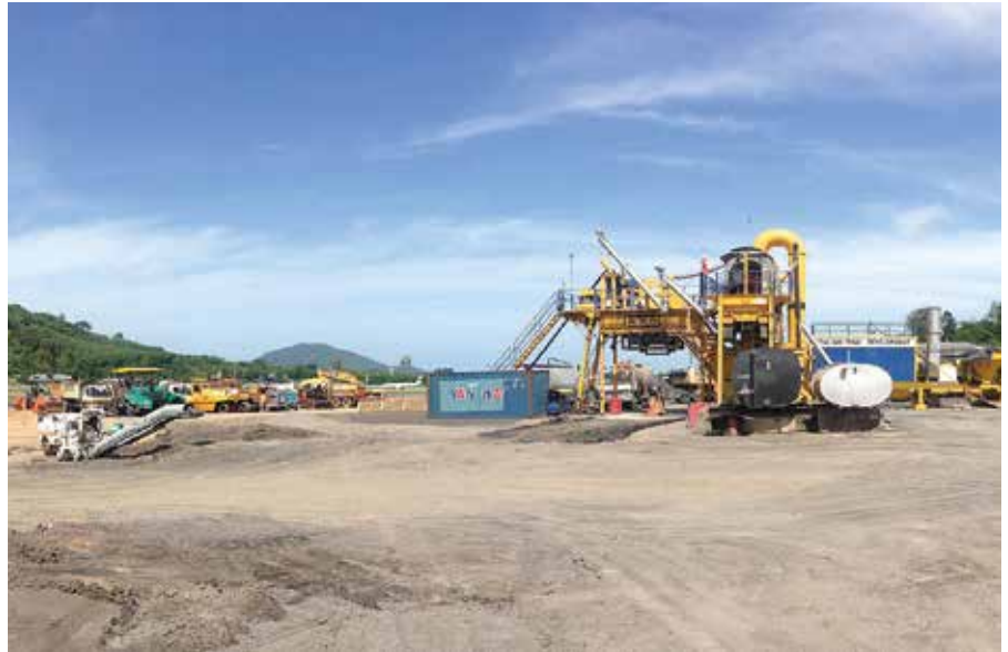
Above and left: Linnhoff's TSD series asphalt plant is highly mobile and versatile. Seen here are two models - the TSD2000 on the runway resurfacing project at the Phuket International Airport (above) and the TSD1000 in the Philippines for local road resurfacing works.
