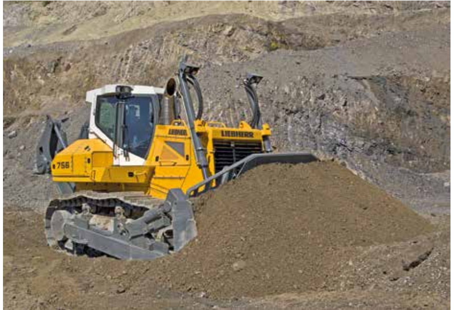
Above: The Liebherr PR 756 Litronic crawler tractor has an operating weight of 38,300 to 41,150 kg and an engine output of 250 kW.
