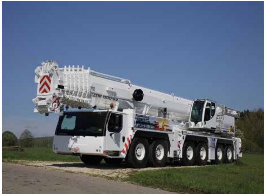
Liebherr's 300 t LTM 1300-6.2 mobile crane on a six-axle chassis made its Asia debut at bauma China.
