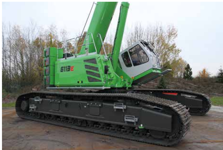
Above and below: The Sennebogen 6113 has a maximum reach of 67 m and safe working load of 120 t.
