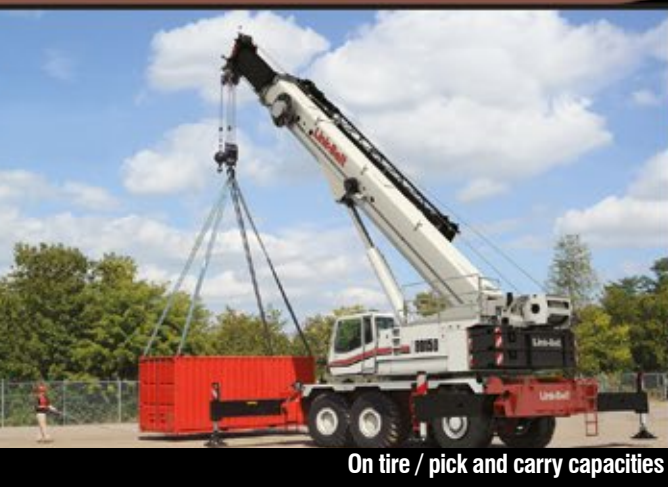
Transport height less than 4.45 m on trailer and less than 3m wide WITH tires and boom
