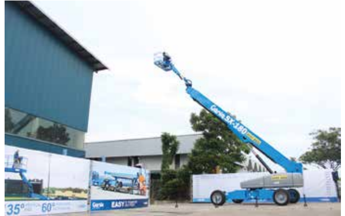
The Genie SX-180 self-propelled telescopic boom lift has a 54.9 m vertical reach and 24.4 m horizontal reach, with a maximum working height of 57 m.
