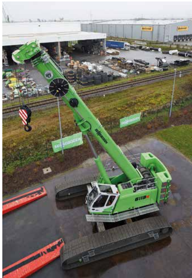
Above and below: The Sennebogen 6113 has a maximum reach of 67 m and safe working load of 120 t.
