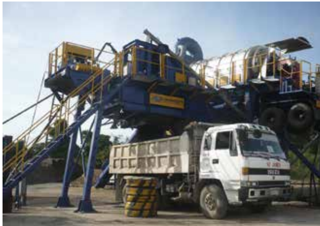
Above and left: Linnhoff's TSD series asphalt plant is highly mobile and versatile. Seen here are two models - the TSD2000 on the runway resurfacing project at the Phuket International Airport (above) and the TSD1000 in the Philippines for local road resurfacing works.
