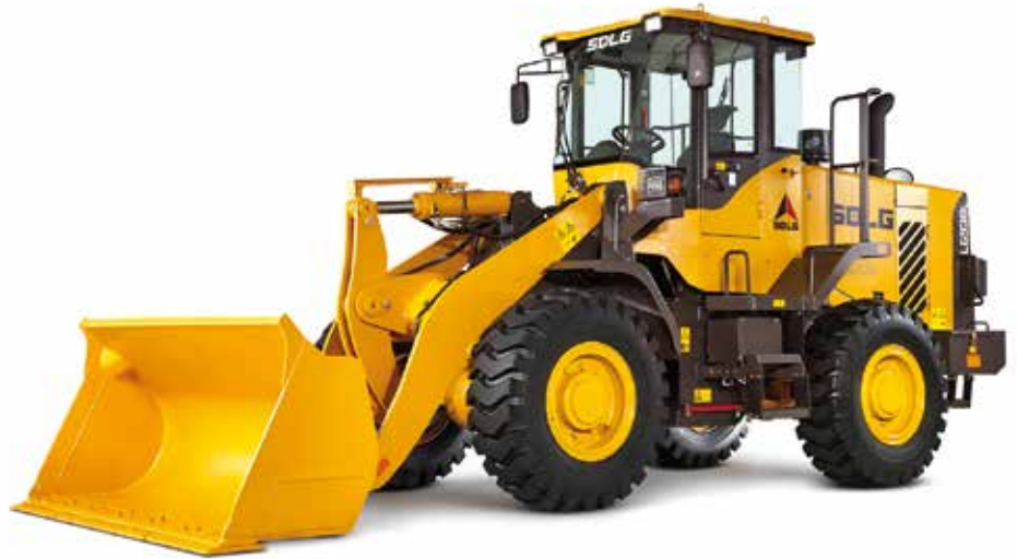
The 3 t capacity LG938L wheel loader is one of SDLG's most popular machines in the international marketplace. With its higher end design specifications, this machine is ideal for construction, mining and aggregates applications.
