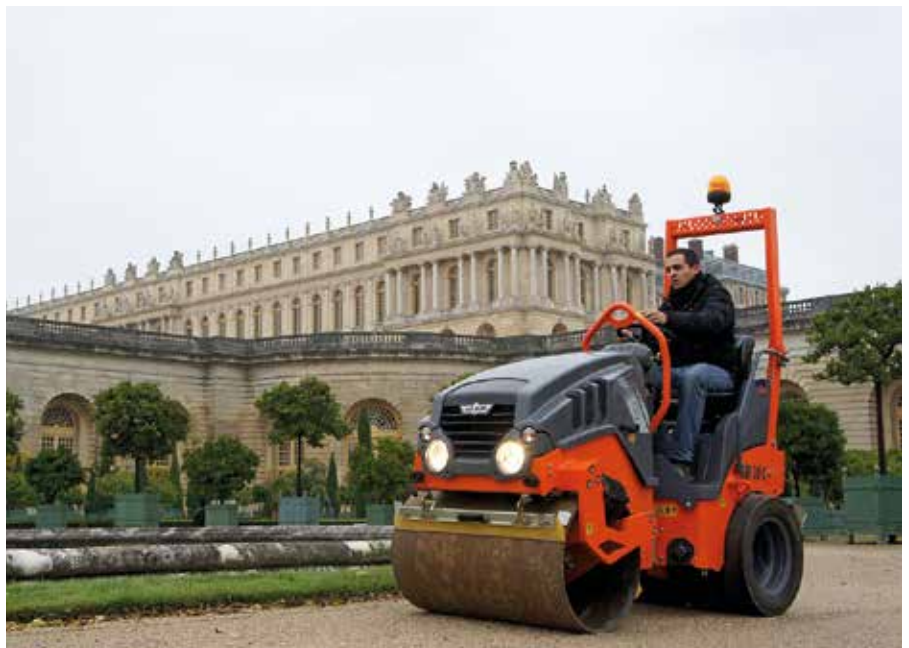
The Hamm HD 10C VT combi roller is an ideal solution for compacting water-bound path surfaces.
