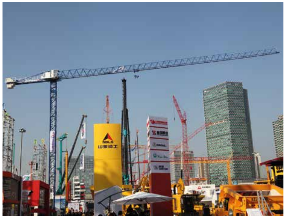
Comansa Jie’s new 11CJ132-6t flat-top tower crane is the first model in the CJ1100 series. Featuring a maximum load capacity of 6 t, it is the smallest model from Comansa Jie to date, with which the company expects to gain market share in countries such as China, India and the Southeast Asia region.
