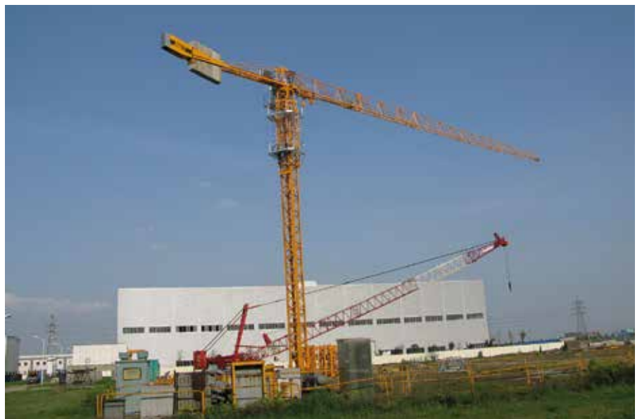
The Potain MCT 85 features a 5 t maximum capacity and an ability to lift 1.1 t at its jib end of 52 m.
