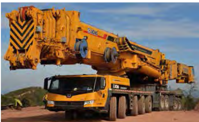
Left and above: The XCA5000 erects a 2 MW wind turbine.
