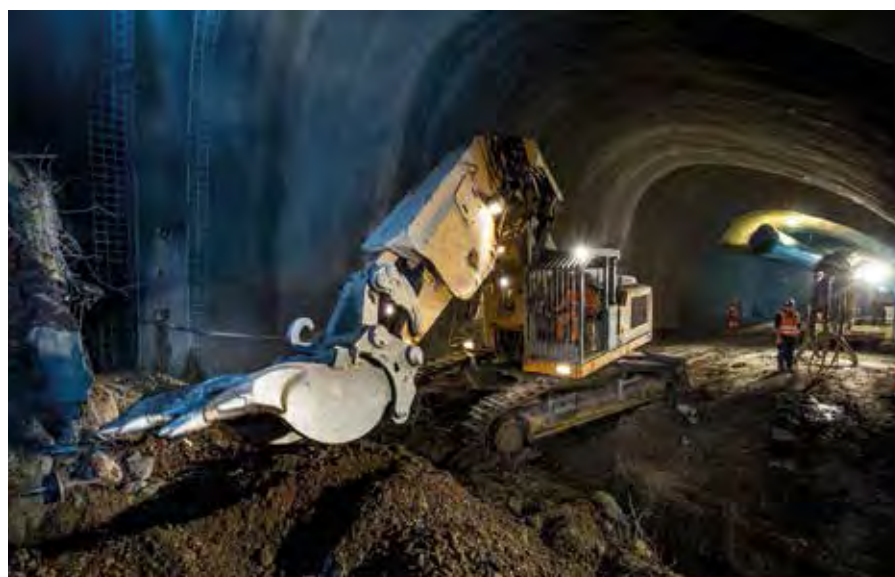
With its 3.07 m long swing arm, the Liebherr R 944 C Tunnel crawler excavator has a maximum tearout force of 164 kN and a maximum breakout force of 191 kN.
