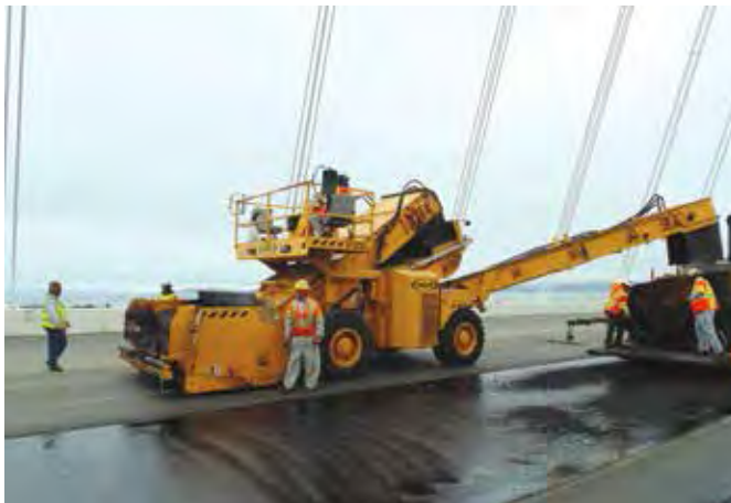
Left and right: The Weiler E1250A remixing transfer vehicle features a conveyor swing, which enables offset paving, and weighs less than an RTV with storage - a key feature when working on bridges.
