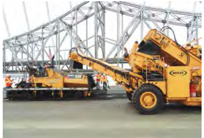
Left and right: The Weiler E1250A remixing transfer vehicle features a conveyor swing, which enables offset paving, and weighs less than an RTV with storage - a key feature when working on bridges.
