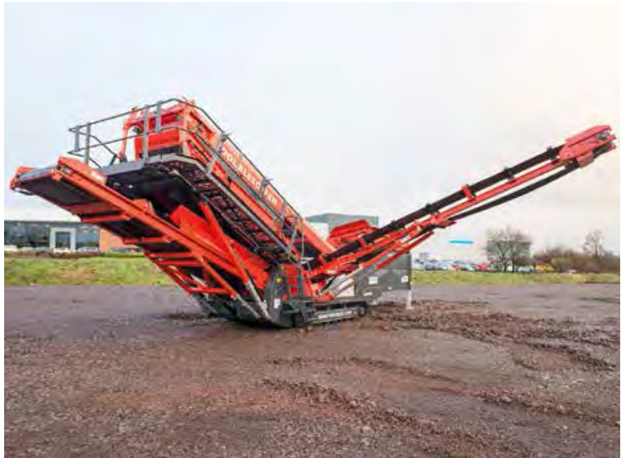
The new Sandvik QA335 Doublescreen has many innovative features, including a user-friendly electrical control system with sequential start up, hydraulic screen separation to aid screen media changes and a fuel efficient 74.5 kW engine.
