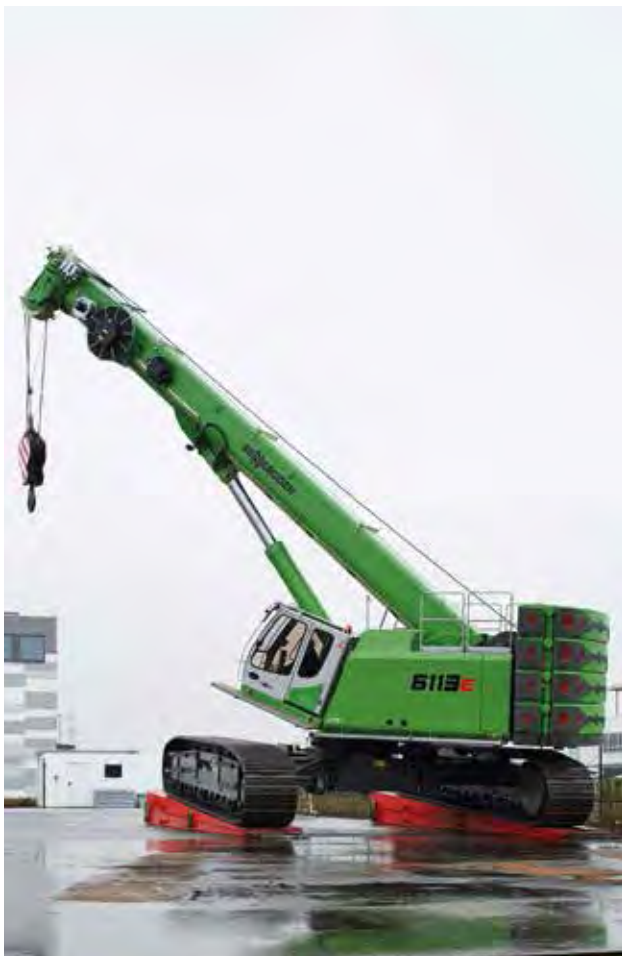
The 6113 is Sennebogen's biggest telescopic crawler crane.
