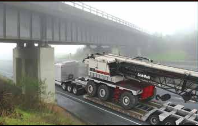
Transport height less than 4.45 m on trailer and less than 3m wide WITH tires and boom
