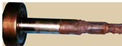
A cast 304 stainless steel impeller mounted on a 403 stainless steel shaft (the shaft is heavily corroded).
