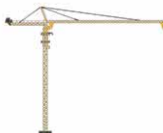
◦ Tower cranes (4-100 ton)
