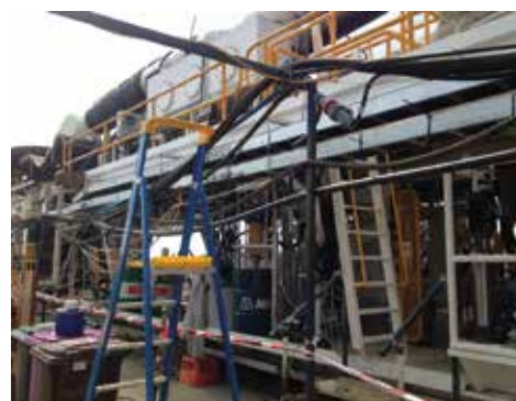
All images: TBM technology is being deployed to build two drifts at the Grosvernor coal mine. Here, Mapei admixtures have also been used for backfill grout.
