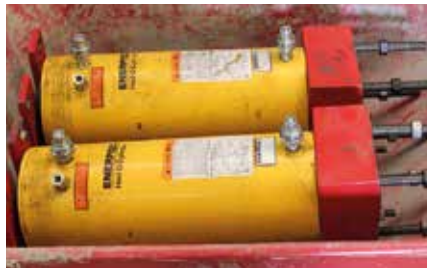
Left: Pulling power for the skidding operation was provided by pairs of RR series double-acting Enerpac RR 3014 cylinders with 368 mm strokes.
