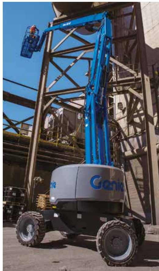
The SX-150 telescopic boom lift (above) and Z-62/40 articulating boom lift.
