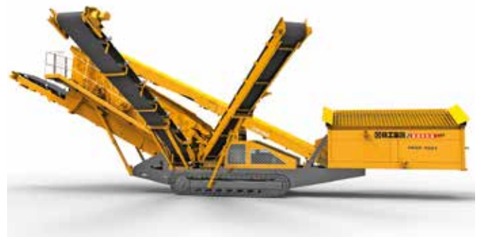
Above: The MSP1561 crawler sieving station has a minimum ground clearance of 343 mm.
