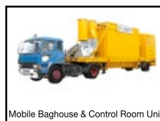
Mobile Baghouse & Control Room Unit
