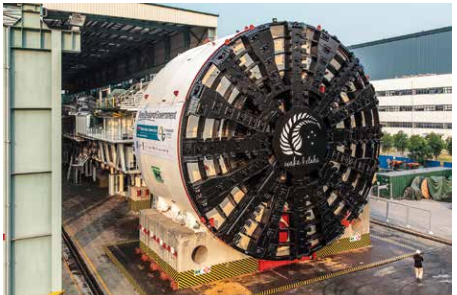
The EPB Shield S-764 was assembled at the Herrenknecht plant in Guangzhou, China. Core components such as the main drive, hydraulic station, electrical station and air locks were manufactured at the company's headquarters in Germany.
