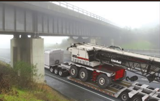
Transport height less than 4.45 m on trailer and less than 3m wide WITH tires and boom
