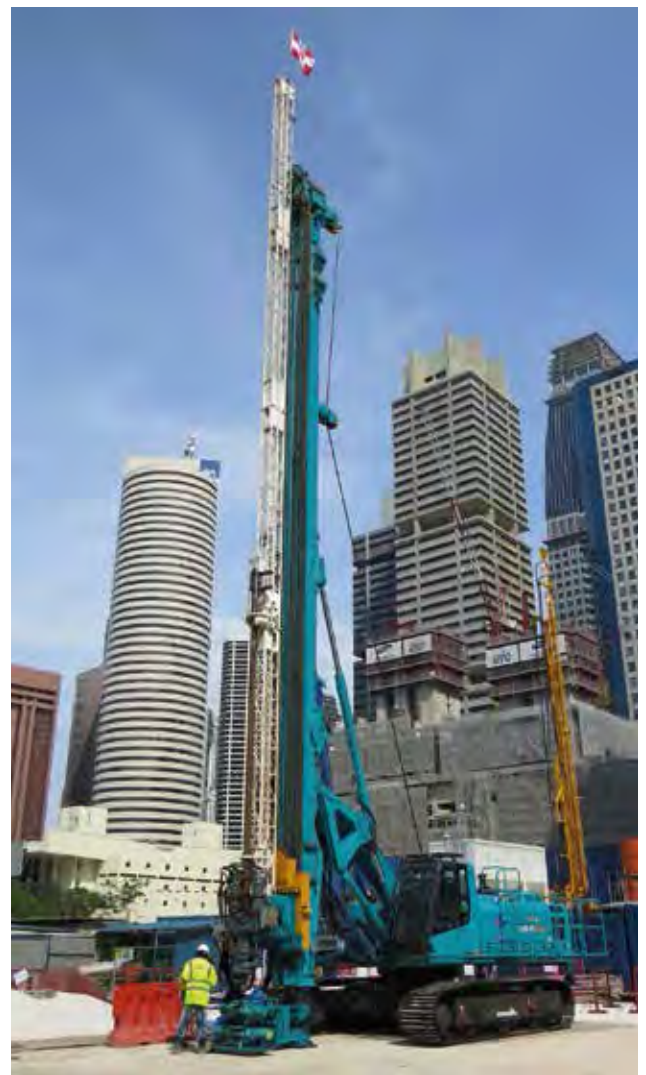
JP Nelson has recently delivered a Sunward jet grouting rig with high pressure pump, mixer and silo system to Shanghai Tunnel Engineering Co Ltd for use in the Thomson Line T225 project.
