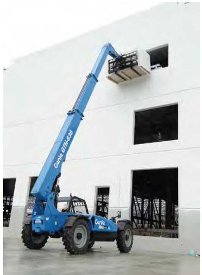
The Genie GTH-636 telehandler has a maximum lifting height of 36 ft and a forward reach of 21 ft 11 in.
