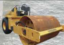
Vibratory Roller Volvo SD100D (10 Ton)
