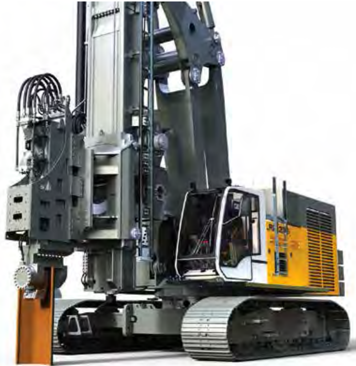
The LRB 355 rig fitted with vibrator.
