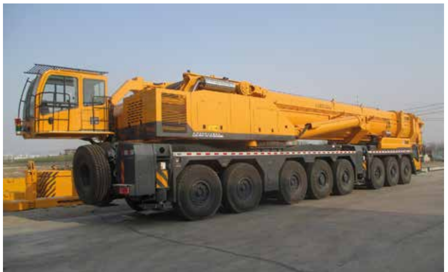
Above, left and right: To cope with the challenge, the construction team employed an XCMG QAY500 all-terrain crane with a maximum lifting capacity of 500 t.
