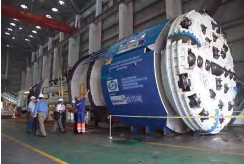
Three 5.23 m diameter Robbins Main Beam TBMs excavated up to 657 m per month in Malaysia.
