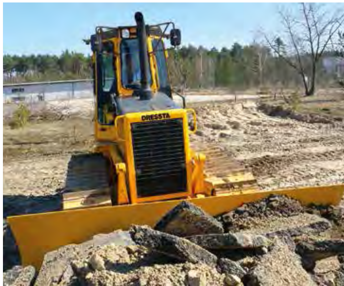
Dressta TD9 hydrostatic crawler dozer.
