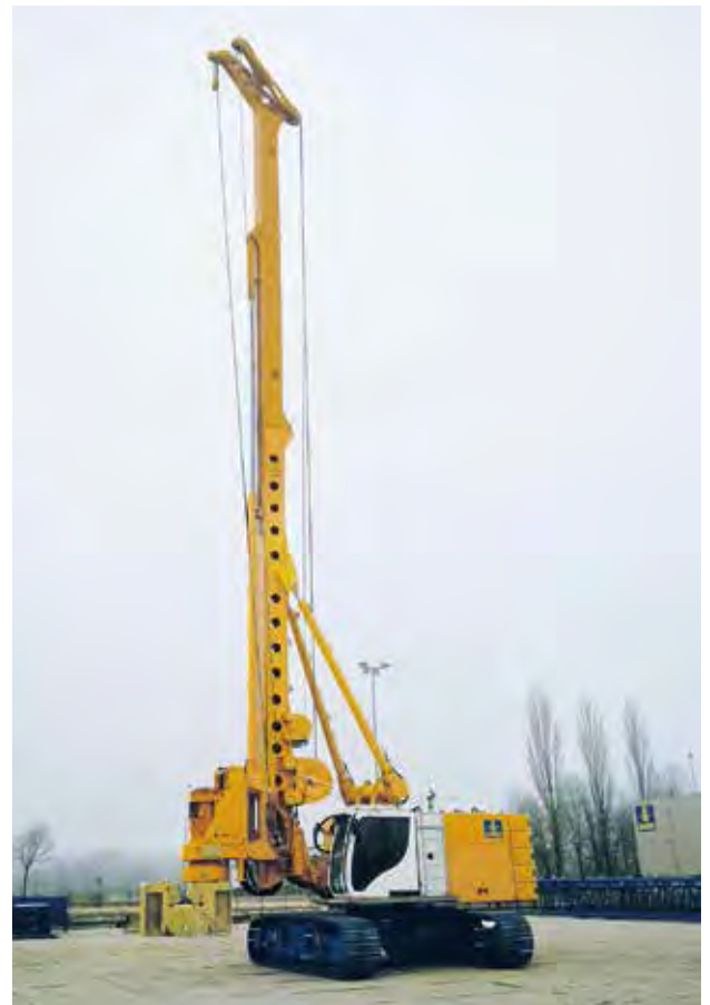
Bauer BG 30 ValueLine rotary drilling rig.
