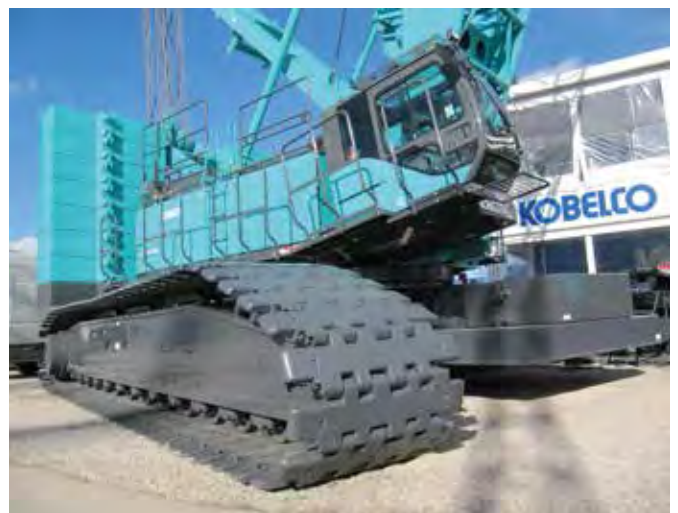
Kobelco CKE2500G crawler crane.
