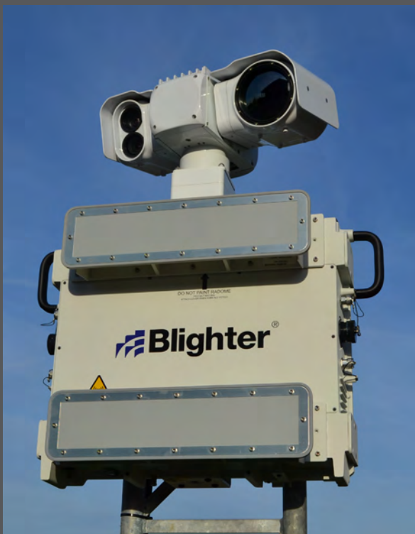
Figure 3 – 90 degree e-scan radar with co-mounted thermal camera system
