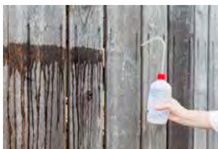
Weathering test: these boards were left outdoors for 17 years. The surface of the untreated board (left) is now so porous that water penetrates it immediately. On the board beside it, on the other hand, the water rolls off in beads. The boards treated with SILRES® WH are still protected by the silicone resin's water repellency. Photo: Wacker Chemie AG
