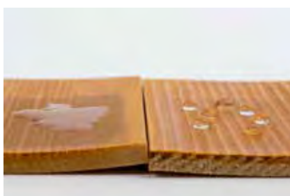
Spruce boards after 1,000 hours of exposure to UV-B light. The board on the right was treated with a wood stain containing SILRES® WH. The wood stain exhibits pronounced water repellency, which causes the water to form beads on the surface that roll off. Photo: Wacker Chemie AG
