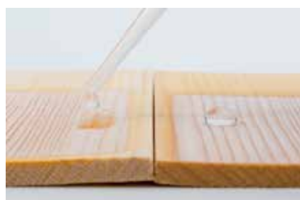
The water repellency of SILRES® WH is still intact, even after 2,000 hours of artificial weathering. The wooden board on the right, which has been impregnated with the silicone resin, is just as protected as before: the water forms beads that roll off. This is not the case with the untreated board (left): the water spreads on the surface and penetrates into the wood. Photo: Wacker Chemie AG
