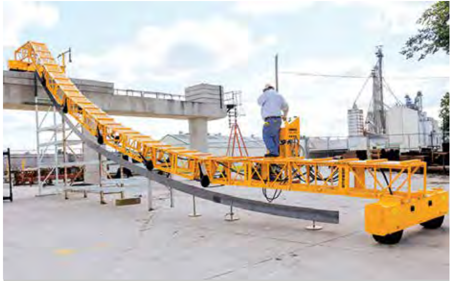
The Gomaco 4000 series Spanit work bridge is fitted with large turnbuckles that can be used to make manual slope adjustments.
