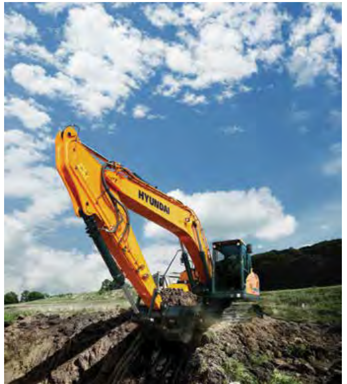
Top and above: The new Hyundai HX220 L crawler excavator can offer a reduction in fuel consumption of up to 12 percent, depending on the type of operation, compared to the 9A-series.
