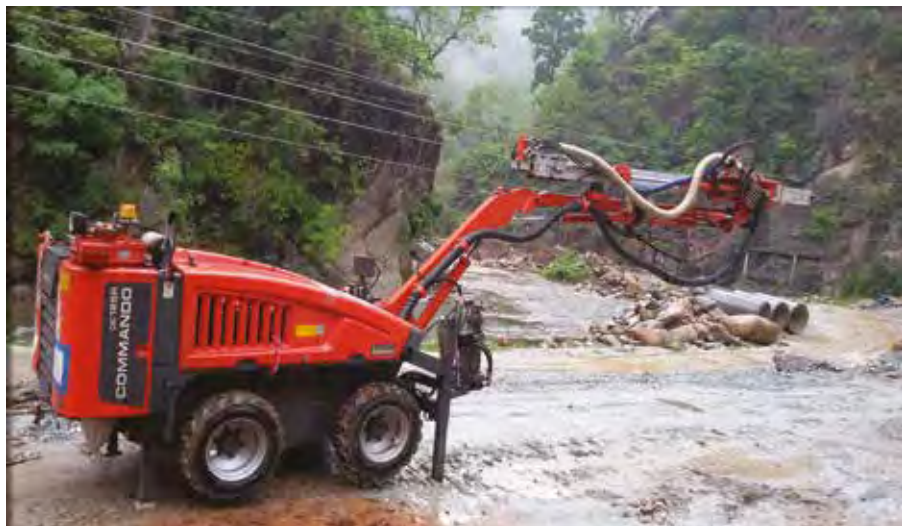
Above: Sandvik's Commando DC125R surface drilling rig on a Nepal hydropower project.
