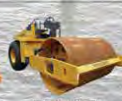
Vibratory Roller Volvo SD100D (10 Ton)
