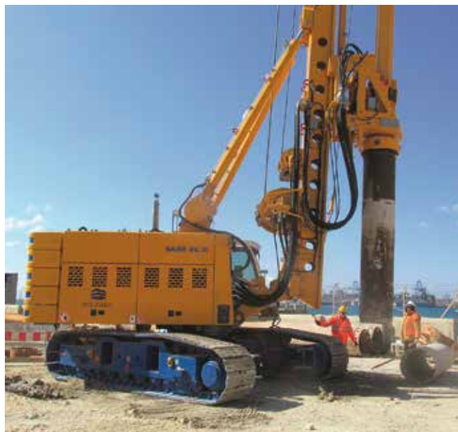
Bauer's ValueLine medium-sized platform series includes BG 26 and BG 30 drilling rigs. The core element is the common base unit BT, which was developed by Bauer.
