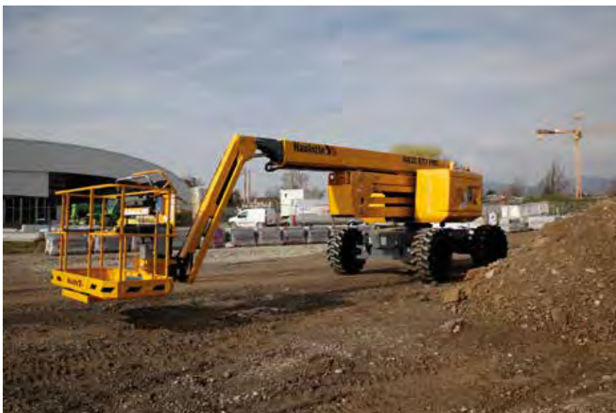
The HA20 RTJ PRO articulated boom can manoeuvre easily on rough terrains.
