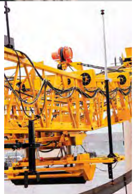
Below: A mast with a Leica Geosystems 3D prism and a slope sensor are used to control the rear 'smart' cylinder's vertical adjustments.
