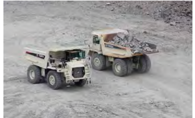
Top and above: Davis Granite uses Terex rigid dump trucks to haul its stone from the pit to the crusher.
