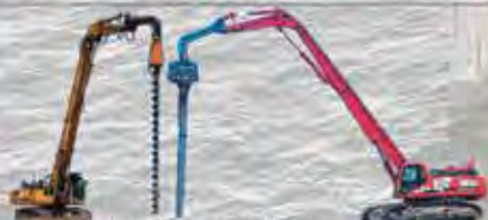
Excavator Auger / Vibro
