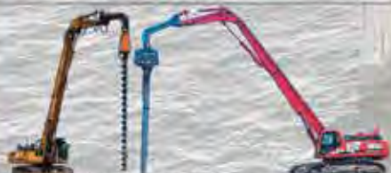
Excavator Auger / Vibro
