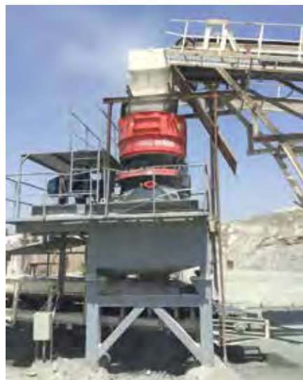
Above: National Quarries in the UAE is also using a Sandvik CH660 crusher.
