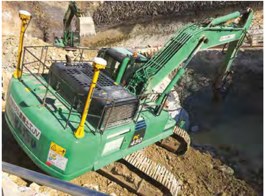
Above, left and below: Tomijima equipped five excavators and five dozers with the Trimble GCS900 Grade Control System. The company has also utilised four Site Positioning Systems Essentials Kits and deployed Trimble SPS620 total stations to conduct high accuracy structural works and checks. Plus, it adopted VisionLink site productivity technology from Trimble for a holistic view of the project site and to track site productivity and materials movement.
