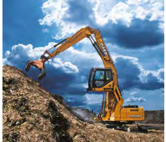
Case CX290D material handling crawler excavator.
