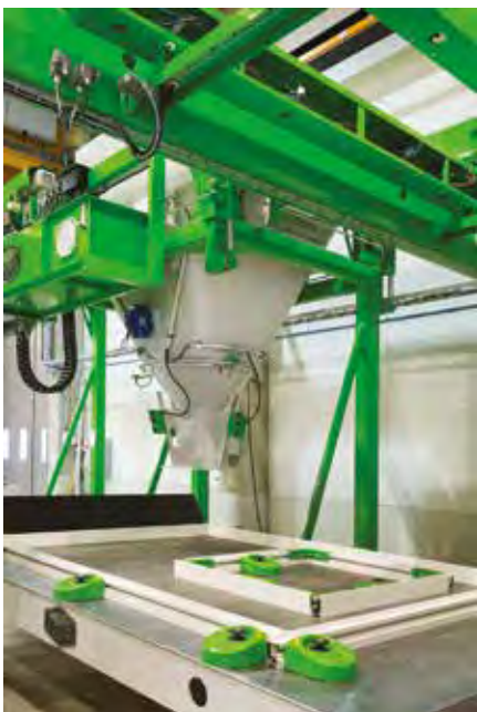
Elematic automated casting machine.
