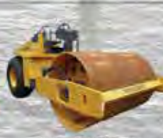
Vibratory Roller Volvo SD100D (10 Ton)
