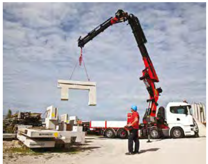
Palfinger PK 165.002 TEC 7 crane can be mounted on a 32 t chassis.
