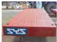
CHECKERED BEAM PLATFORM FOR TEMPORARY ACCESS
