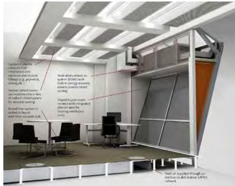
Above: An overview of the systems installed in the 550 sq m 3for2@UWCSEA pilot project.
