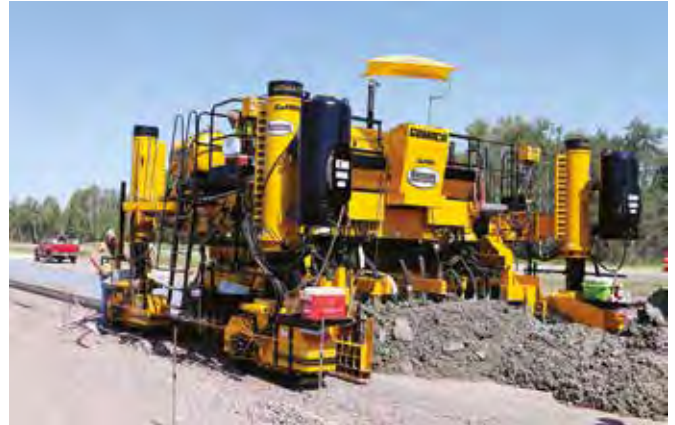
Gomaco GP3 slipform paver.
