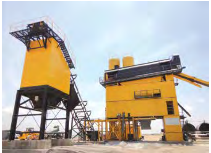
Above: A Lintec CSD3000 containerised asphalt plant was used on the track resurfacing project at the Sepang International Circuit.
