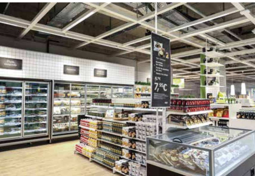
In the Swedish shop LVT floorings were bonded with ULTRABOND ECO V4 SP, after priming the substrates with ECO PRIM T and smoothing with MAPESOL 3.
