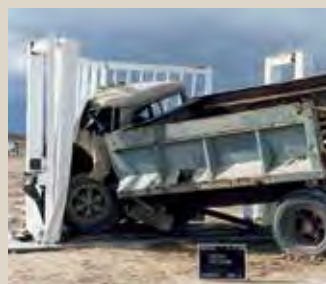
TT280 High Security Linear Crash Gate
