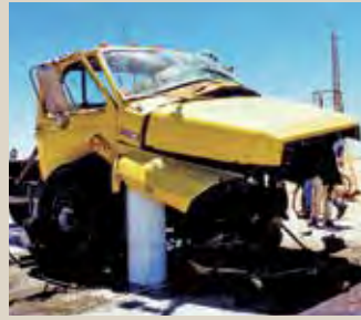
DSC720 High Security Bollard
