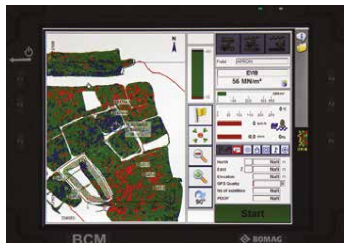
Above and right The BCM 05 compaction control system and the Bomag GPS system ensure that the daily compaction checks required are documented smoothly.
