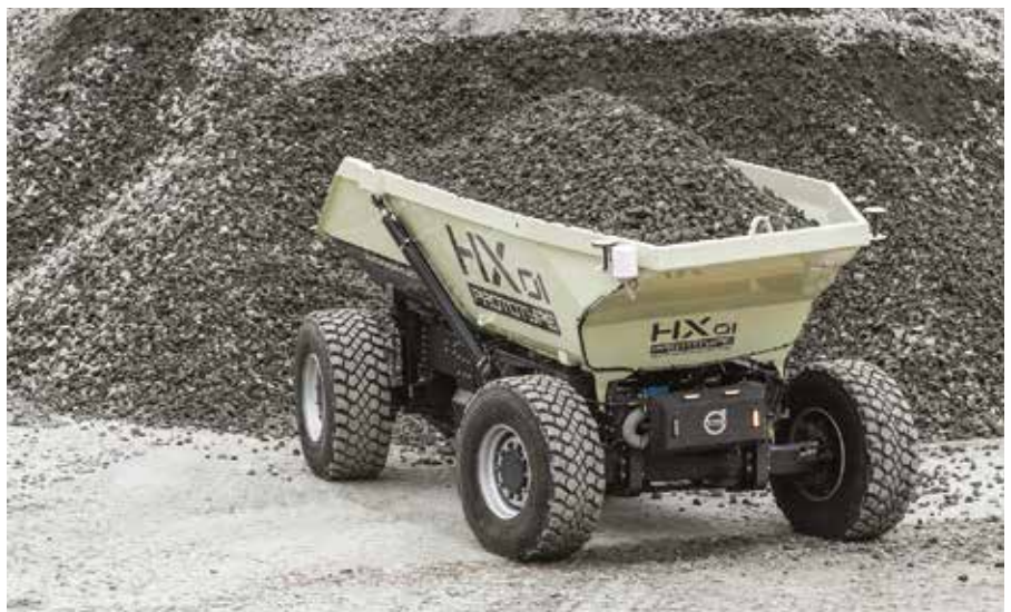
Top and above: The Volvo HX1 prototype autonomous, battery electric, load carrier is part of a research project that predicts up to a 95 percent reduction in carbon emissions and up to a 25 percent reduction in total cost of ownership.
