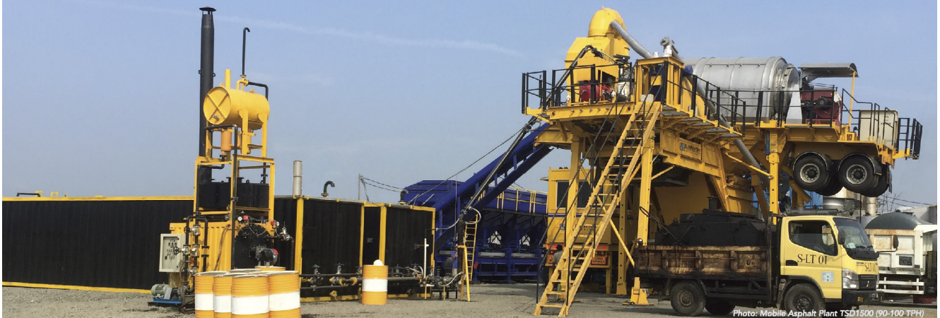
Photo: Mobile Asphalt Plant TSD1500 (90-100 TPH)
