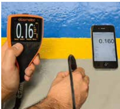
Transfer data to PC or mobile devices via Bluetooth or USB.
