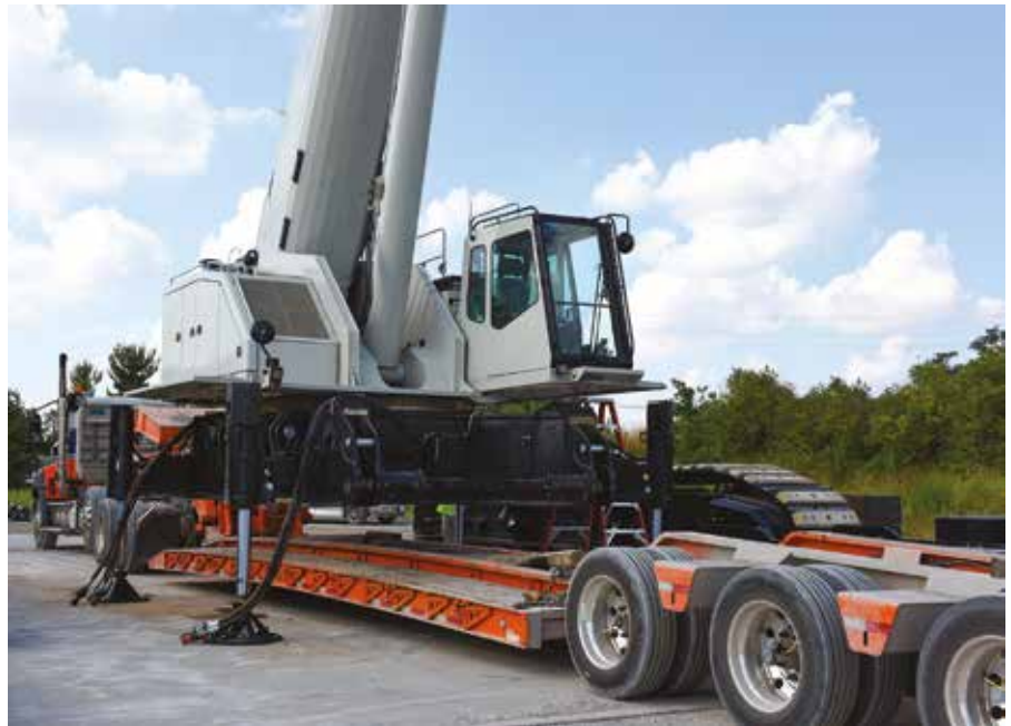
Top and above: The new Link-Belt TCC-2500 telescopic crawler crane.
