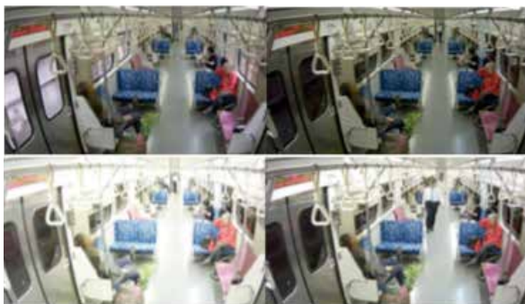
Fig. 1: Video captured from traditional onboard camera when entering a tunnel.
