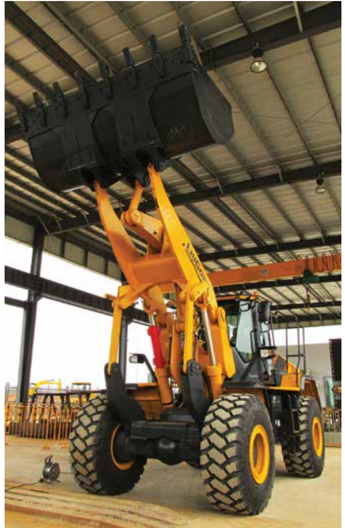
Compared to conventional radial lift wheel loaders such as the 856H (left), the VL wheel loader (above) is more fuel-efficient as it allows more tons material to be moved per horsepower.
