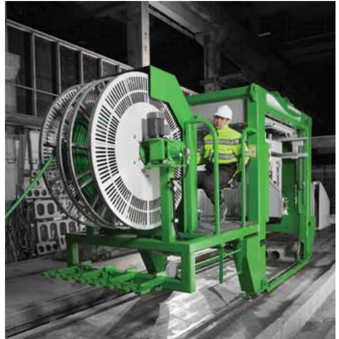
Above and below: The Sawpreparer S5 (above) and Extruder S5 are two of the key equipment in the Semi Floor production line.
