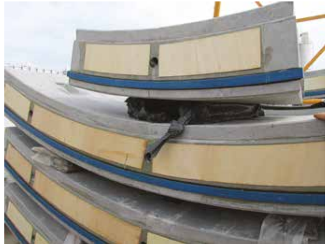
Above and left: The tunnel linings are made of steel fibre reinforced concrete (above), making them more durable and fire-resistant.
