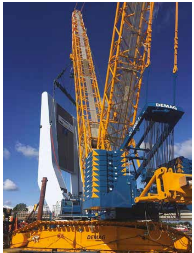
Below: The massive 30.7-m-long bridge segments required LSL_2 configuration with 60 m of main boom for the CC 3800-1 crane and 36 m Superlift mast. The 165 t counterweight on the crane's superstructure, 50 t central ballast and 325 t on Superlift tray were necessary to give the crane a 347-t capacity when working at the predetermined fixed 24-m radius.
