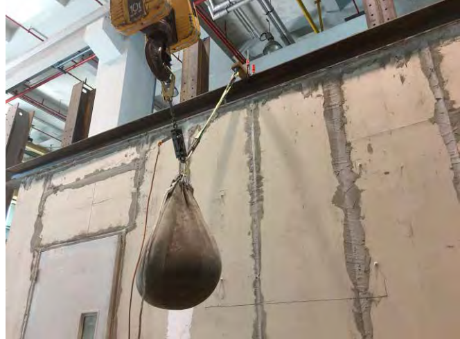
Conducting a door slam test at PSB. Photo: © Vodapruf
