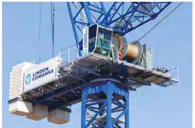
Below: The hoist motor of the crane allows speeds of up to 170 m/min.
