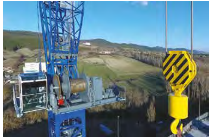
Above: The new LCL700 features a high-capacity hoist cable drum that enables the crane to construct buildings of over 1,000 m in height.
