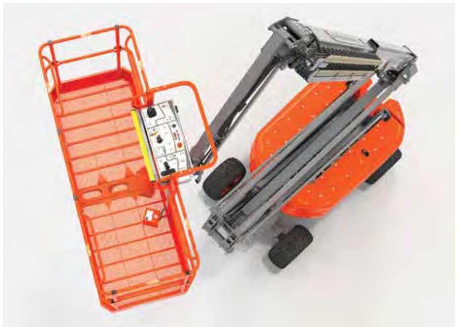
Top and above: The new Skyjack SJ85AJ articulating boom lift features dual platform capacities of 340/227 kg and three/two personnel rating. It delivers a working height of 27.91 m, platform height of 25.91 m, horizontal outreach of 17.07 m and an up-and-over clearance of 10.36 m.
