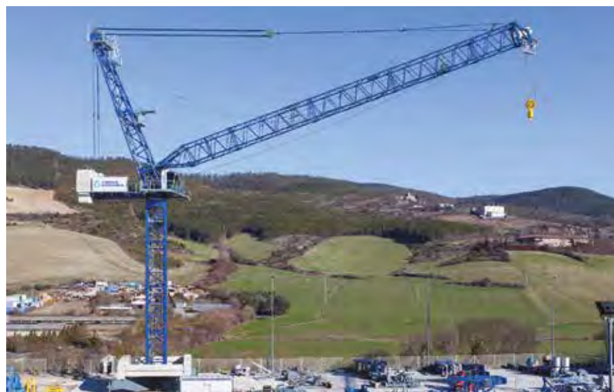
The maximum reach of the new LCL700 is 65 m. The prototype in this image has been assembled with a 45 m reach.
