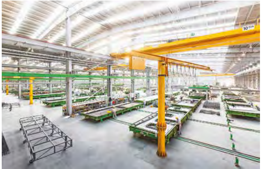
Elematic sandwich wall production circulation line.
