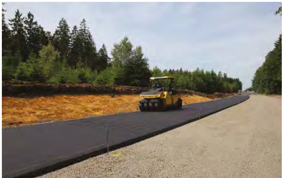
Above and below: The new Bomag BW 28 RH pneumatic tyred roller features a large 3 cu m ballast compartment and efficient weight ballast changing system. The machine is suitable for a wide range of applications, from city streets and county roads to highways and airports.
