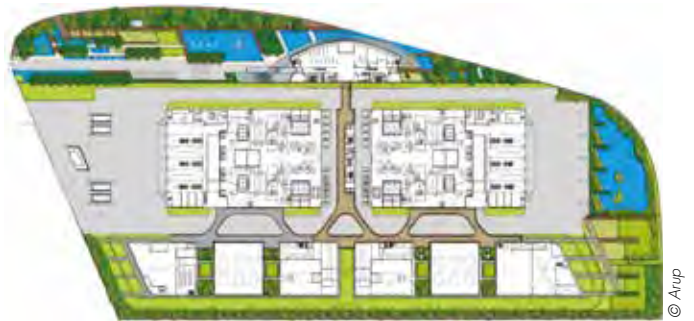
Above: The floor plan of the two-mirror image main process buildings, housing identical processes.
