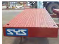
CHECKERED BEAM PLATFORM FOR TEMPORARY ACCESS
