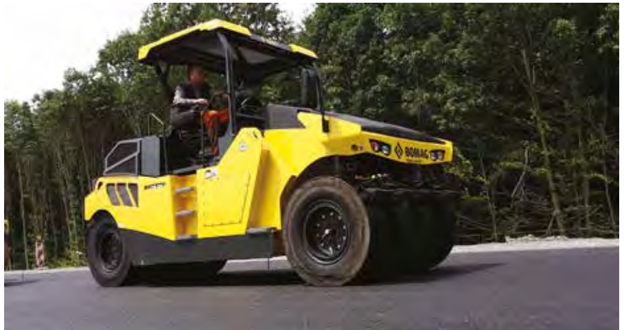
Above and below: The new Bomag BW 28 RH pneumatic tyred roller features a large 3 cu m ballast compartment and efficient weight ballast changing system. The machine is suitable for a wide range of applications, from city streets and county roads to highways and airports.
