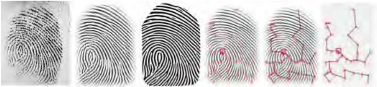
The process of data extraction from a typical fingerprint scan creates an encrypted pattern, no fingerprint image is stored.
