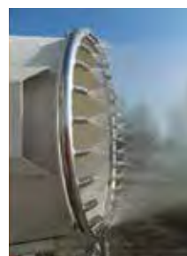
Second image from the top and above: The Dust Fighter DF 7500 is ideal for construction and demolition works. This model has a maximum range of 40 m with a rotation angle of 335°.
