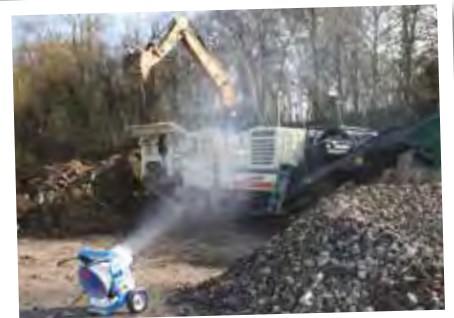
Above and inset: The DF Mini (above) is suitable for indoor use and the DF Smart (inset) is the smallest dust control unit of the Dust Fighter range that can be used for outdoor jobs.
