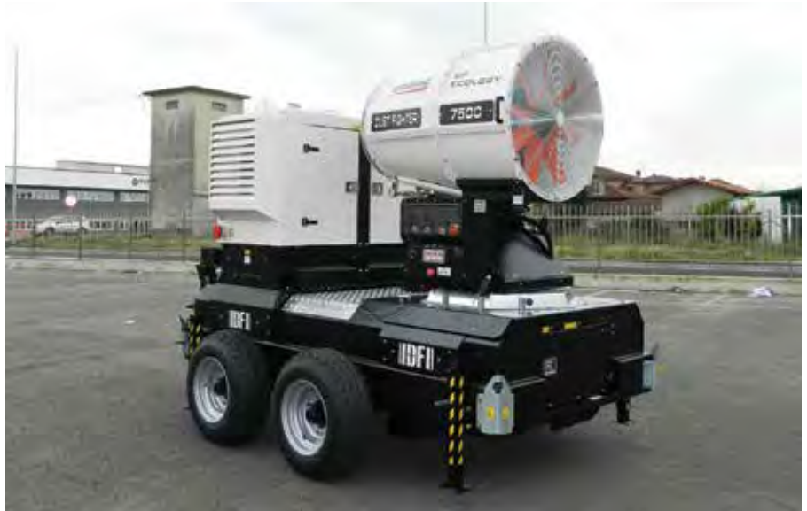
Above: The power supply for the Dust Fighters comes from a generator or electrical mains (left) and the water supply comes from a tank or public water net (right).
