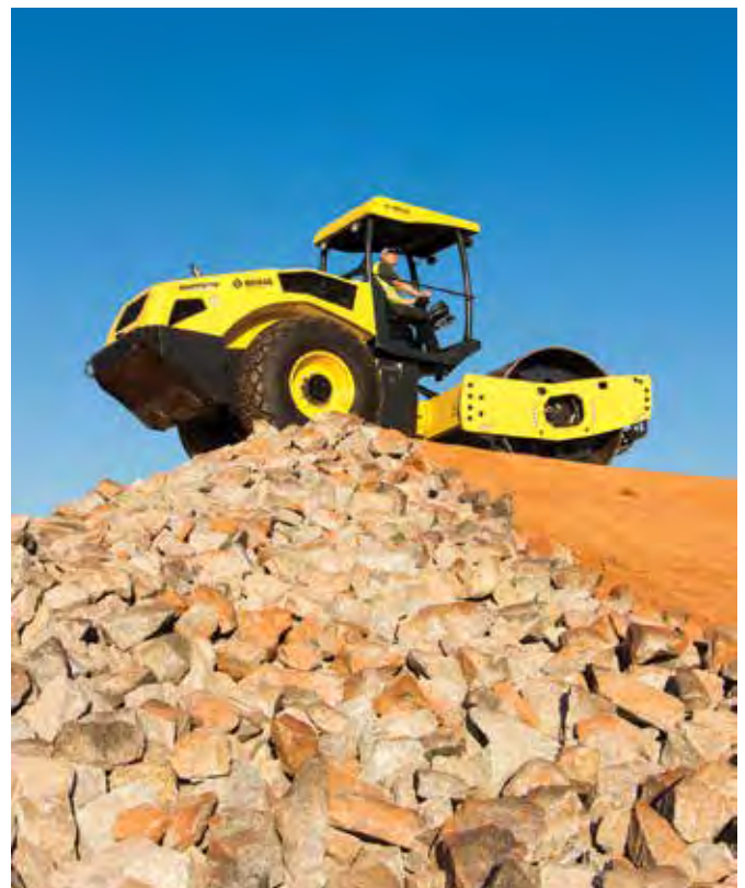
Left and right: The new Bomag BW 211 DH-5 single drum vibratory roller boasts a dual pump drive system, allowing the machine to climb grades as steep as 60 percent.
