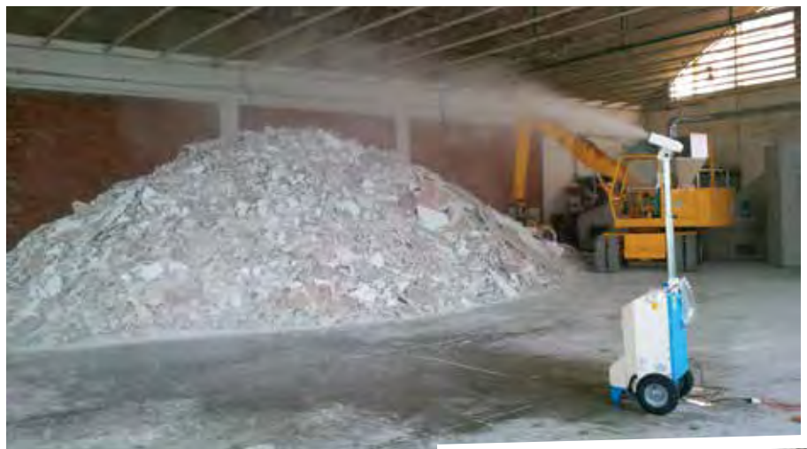
Left: Generac Dust Fighters offer a safer and healthier solution. The nebulised water particles created from these units have a 40-150 micron diameter, so they can easily bond with dust particles of the same dimensions and drive them to the ground.
