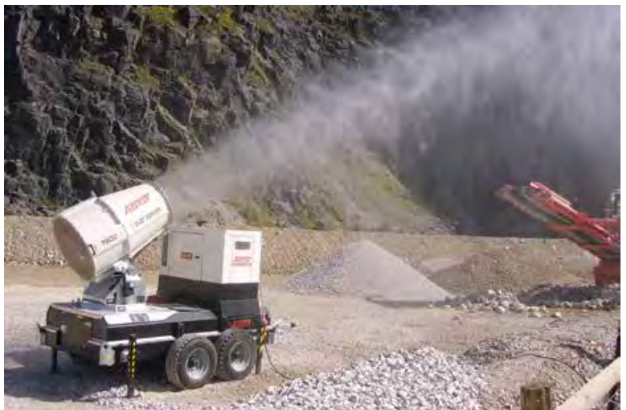
Second image from the top and above: The Dust Fighter DF 7500 is ideal for construction and demolition works. This model has a maximum range of 40 m with a rotation angle of 335°.
