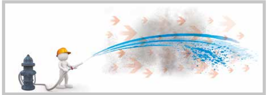
Above: The traditional water-spraying method is considered less efficient. The average size of a dust particle is 80 micron in diameter, while water particles created from a standard irrigation system have a 1,000 – 1,500 micron diameter and are therefore too big and will go through the dust cloud.
