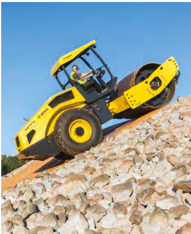
Left and right: The new Bomag BW 211 DH-5 single drum vibratory roller boasts a dual pump drive system, allowing the machine to climb grades as steep as 60 percent.
