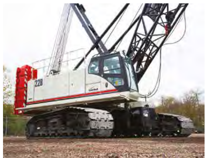
Top and above: The Link-Belt 228 HSL crawler crane offers maximum boom lengths with two different styles of boom: tubular boom, up to 71.6 m and angle boom, up to 47.2 m. The model is also fitted with the 'Eco Winch' fuel saving feature.
