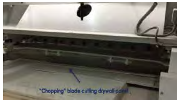
Adopted the use of machines and automated equipment for cutting cementitious panels and Zyclum studs.
