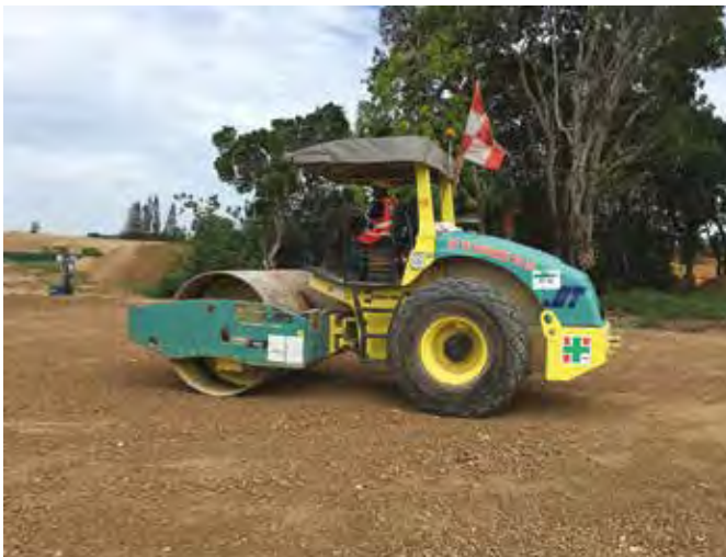
ABOVE AND BELOW: Ammann ASC 110 single drum rollers work on the construction of a new runway at Singapore Changi Airport. The machines are designed with no-rear-axle concept that provides an individual drive for each tyre.
