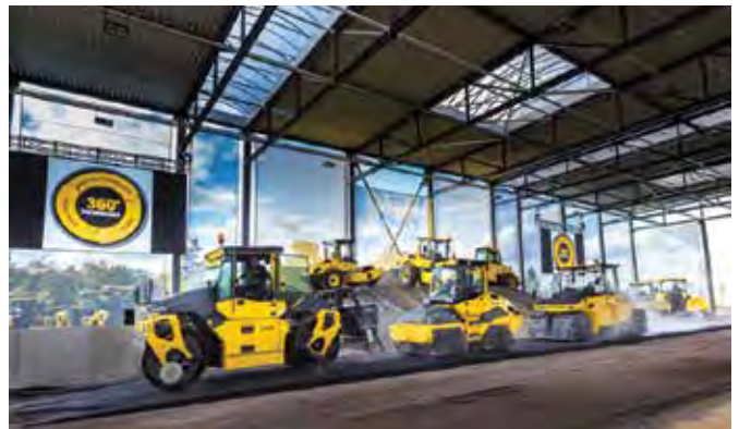
Bomag has introduced several new tandem rollers at the company's Innovation Days 2017, among which were the BW 154 APO and 174 APO with split drums.
