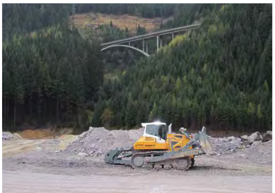
With the hydrostatic drive, the speed of the diesel engine can be kept constant in practical use regardless of the required load. Therefore, the PR 766 crawler tractor always runs at the optimum efficient speed.
