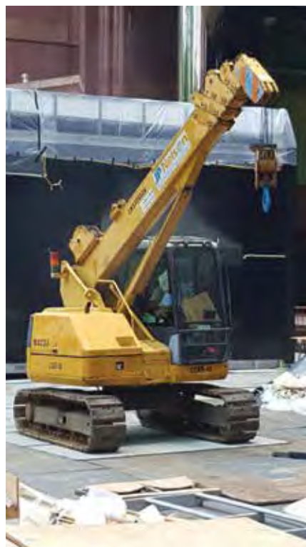
ABOVE, LEFT AND FAR LEFT: Mini cranes can perform lifting tasks on various construction sites. They are also ideal for use indoors or in a tight and narrow areas, where larger cranes are not able to access.
