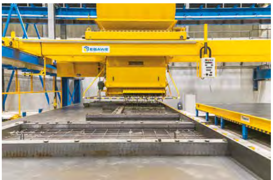
TOP AND ABOVE: Greyform Building, the latest ICPH in Singapore, is a multi-storey advanced manufacturing facility designed for producing prefabricated construction elements, such as precast concrete components, with a high degree of automation.
