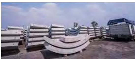
ABOVE LEFT AND LEFT: The tunnel lining rings were assembled at a manufacturing plant for precast concrete segments, and then delivered to the jobsite. Mapei systems were also applied during the production of these lining rigs.
