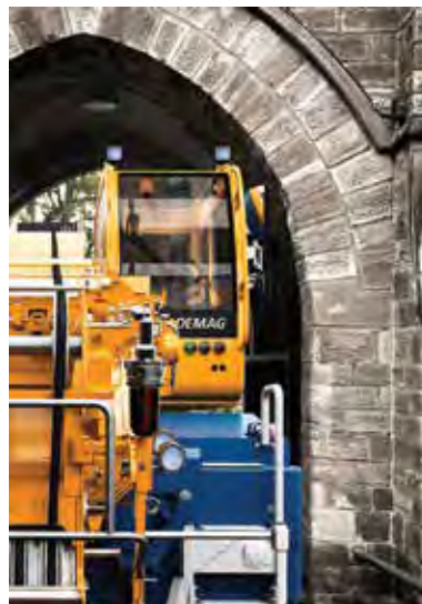
TOP, ABOVE AND LEFT: The new 45-t Demag AC 45 City crane is highly compact with a total length of only 8.68 m, a width of 2.55 m and an overall height of just 3.16 m. It also features a vast configuration flexibility, making it possible to customise the crane perfectly for the requirements at hand.
