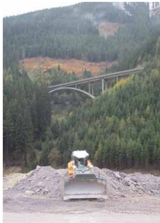
The machine is designed with an oscillating undercarriage, so that the track rollers can be flexibly adapted to the surface. As a result, the machine's traction - and its smooth running - is significantly increased, particularly when used on stony ground.
