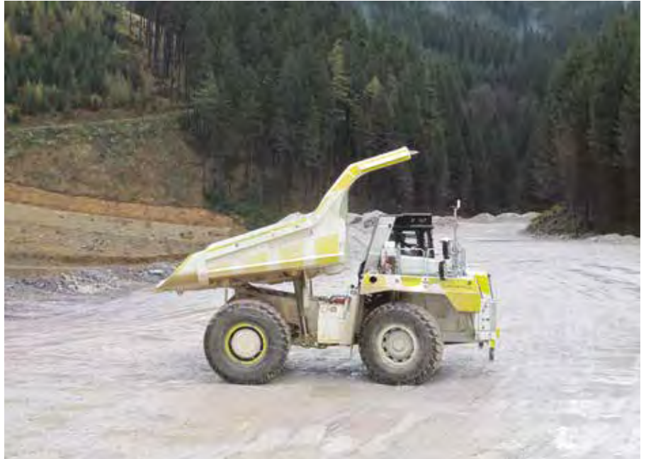
ABOVE AND LEFT: The T 236 is ideal for use at both quarries and mining sites. It is said to be the first diesel electric truck in its class that incorporates oil immersed braking system with four corner retarding capabilities, resulting in reliable braking technology.
