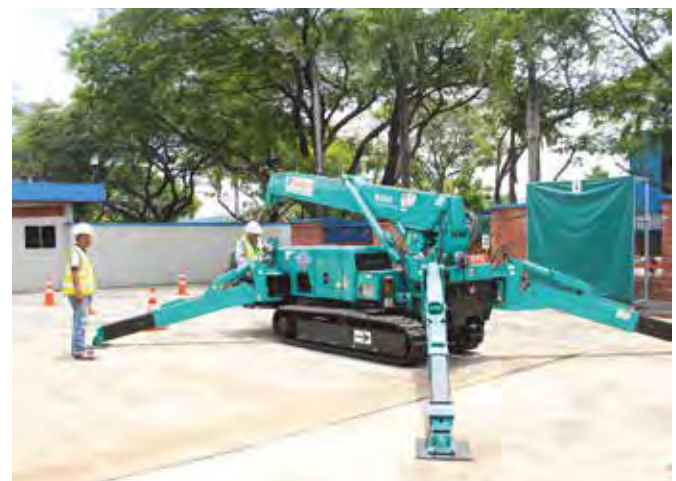
ABOVE AND BELOW: The Maeda MC-405C crane being used for operator training at the JP Nelson facility on Benoi Road. The training programme, covering both theoretical and practical sessions, is aimed to raise the competency of mini crane operators.
