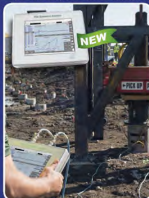
Pile Dynamics Analyzer-Dynamic Load Tester (PDA-DLT) for Drilled Shafts
