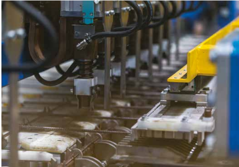
Another part of Greyform Building is a steel reinforcement fabrication plant. Here, the automated steel reinforcement machine allows full flexibility in product customisation to produce steel mesh, stirrup cages, cut and bend reinforcement bars and reinforcing cages.
