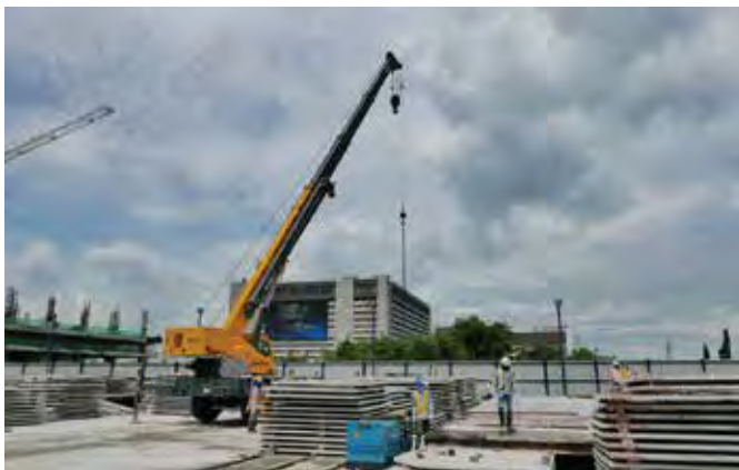
ABOVE AND BELOW: Grove RT530E-2 rough-terrain crane being used by MDC Equipment Solutions at its precast plant in San Felix, the Philippines, to handle concrete sections.
