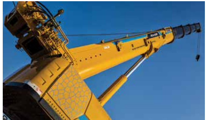
LEFT AND RIGHT: The new XCMG XCA100E all-terrain crane has a maximum lifting capacity of 100 t. The machine is designed with an independent suspension system, four steering modes and a new energy-efficient hydraulic system.
