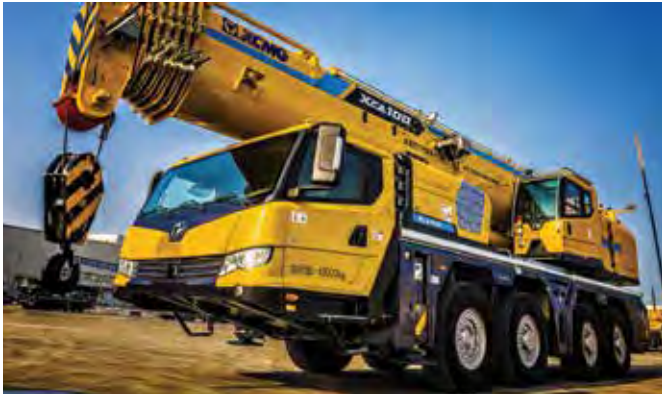
LEFT AND RIGHT: The new XCMG XCA100E all-terrain crane has a maximum lifting capacity of 100 t. The machine is designed with an independent suspension system, four steering modes and a new energy-efficient hydraulic system.
