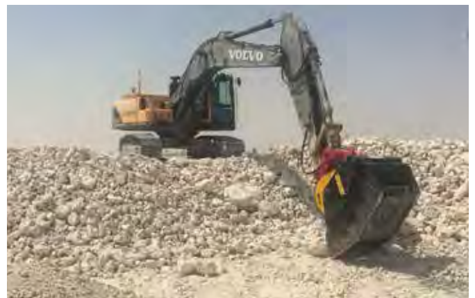
ABOVE: The BF90.3 crusher bucket mounted on a Volvo excavator takes part in the construction of Oryx International School in Doha.
