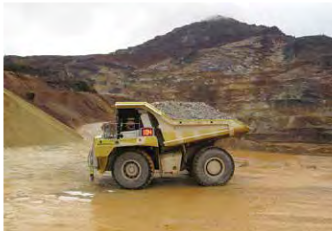
ABOVE AND LEFT: The T 236 is ideal for use at both quarries and mining sites. It is said to be the first diesel electric truck in its class that incorporates oil immersed braking system with four corner retarding capabilities, resulting in reliable braking technology.
