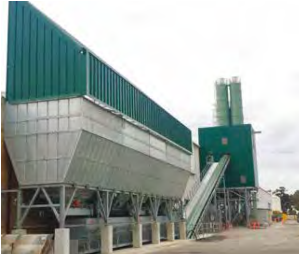
ABOVE AND ABOVE RIGHT: MCT Italy, in collaboration with Bennett Equipment, delivered a special concrete batch plant to Boral specifically designed to produce the concrete for the tunnel segments.
