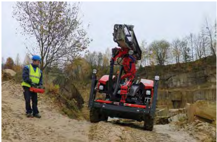
The Commando DC130Ri drill rig features an excellent off-road capability and versatility for vertical and horizontal line drilling. The machine's optimised centre of gravity means it can also reach steep slopes without any problems.
