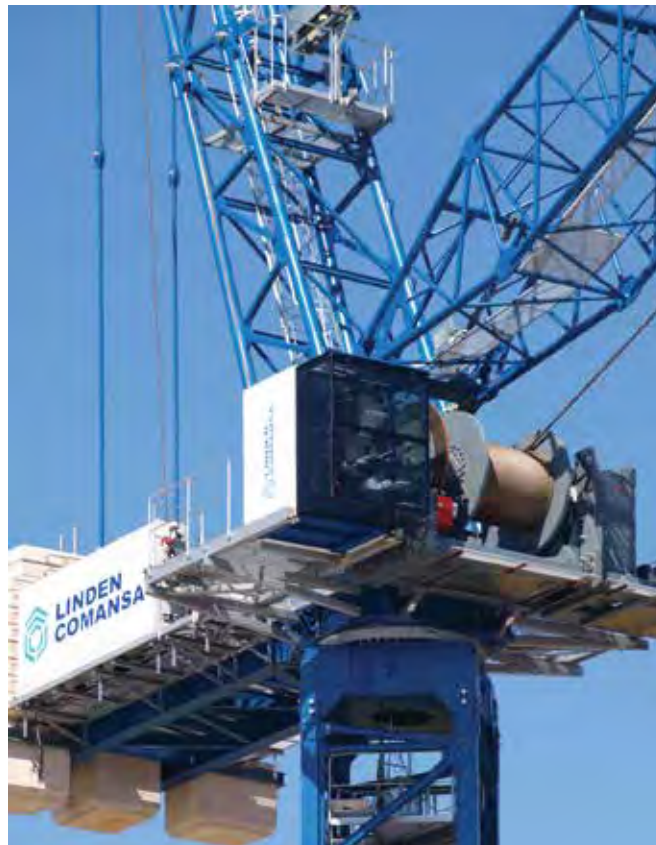
ABOVE: Linden Comansa LCL700 has a minimum reach of just 4 m and maximum reach of 65 m. The model comes in two versions: 64 t and 50 t.
