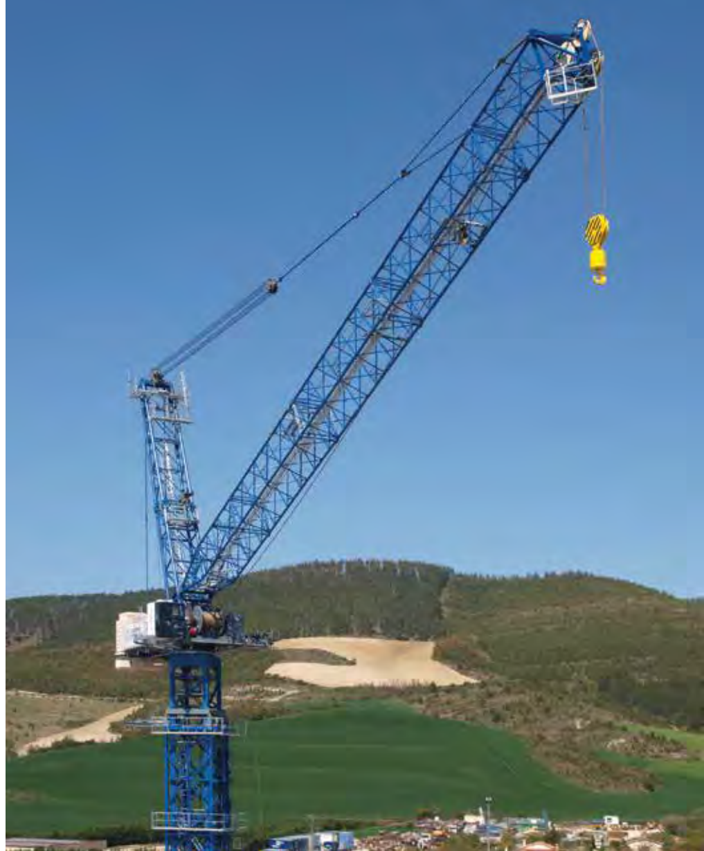
ABOVE: Linden Comansa LCL700 has a minimum reach of just 4 m and maximum reach of 65 m. The model comes in two versions: 64 t and 50 t.
