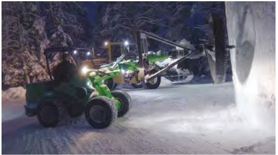
ABOVE, LEFT AND BELOW (LEFT AND RIGHT): Auger Torque helped Avant to design and build a special ice auger and frame to suit the Avant 760i loader. They were used together with the Auger Torque 4500 MAX earth drill to drive through the heavily packed snow and ice wall.
