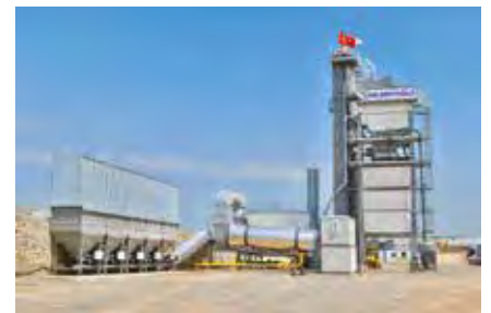
TOP AND ABOVE: Ammann ABA 340 UniBatch asphalt-mixing plant being used by paving company Nalbantoğlu İnşaat to help with the construction of the Northern Marmara Motorway in Turkey.
