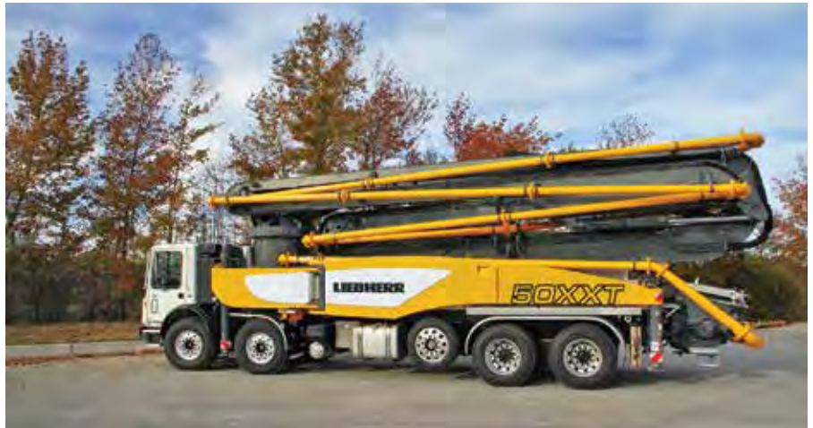
Liebherr 50 M5 XXT truck mounted concrete pump.
