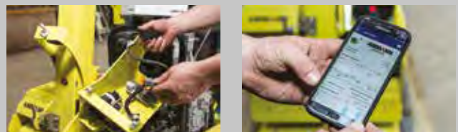
LEFT AND RIGHT: The Ammann ServiceLink provides machine data such as battery status, usage, maintenance intervals and documentation to be accessed via the free Ammann Service App or the Service Portal.
