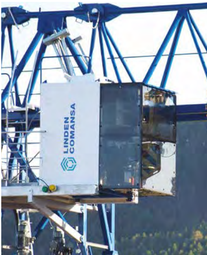
TOP AND ABOVE: The CUBE cab is available in two sizes - L and XL - and fitted as standard on most of Linden Comansa’s tower cranes.
