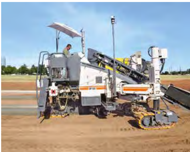
Wirtgen SP 62i (above) and SP 15i slipform pavers.
