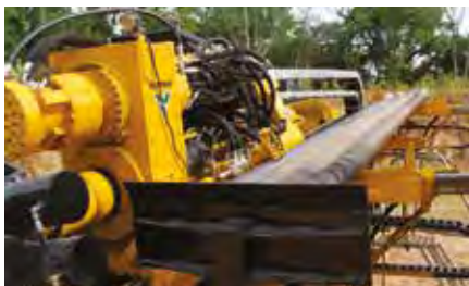
BELOW LEFT: The D220x300S is able to stage five rods at one time, increasing boring efficiency by minimising rod loading time.
