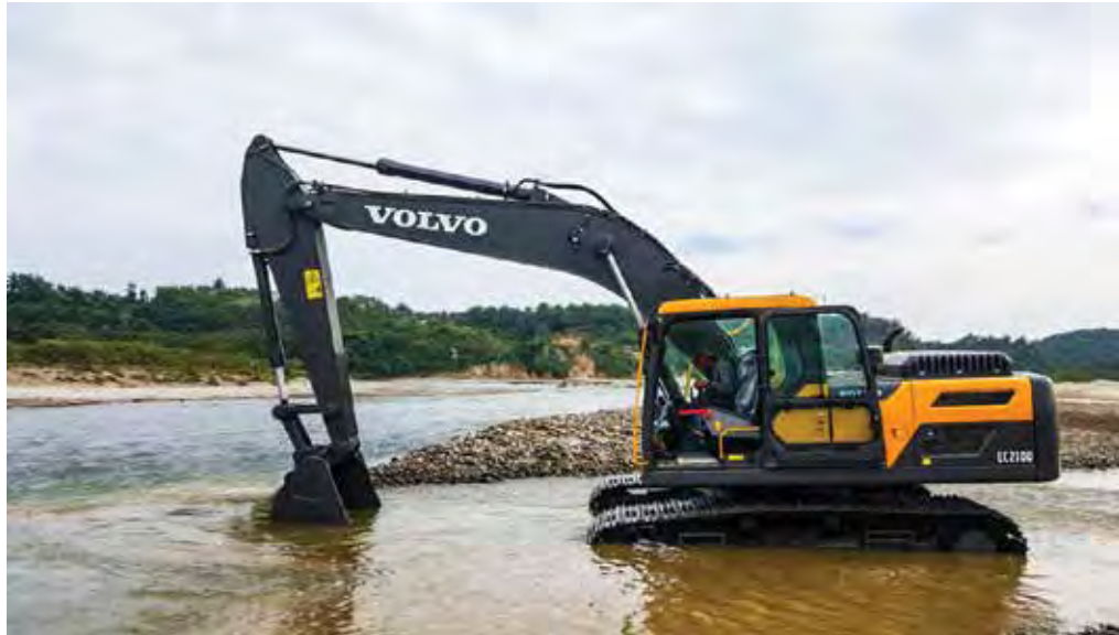
Volvo EC210D excavator works for CV Ocbama Group to extract material from the Seblat River in Bengkulu. The machine is loading up to 500 cu m of rock per day, which will later be processed for use in construction projects in the surrounding area.
