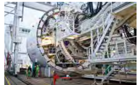
BELOW LEFT, BELOW AND BOTTOM: A total of four TBMs were supplied by Herrenknecht for the construction of new road tunnels under the Suez Canal. The Mixshields with a diameter of 13.02 m created over 15 km of new tunnel for the large-scale project.
