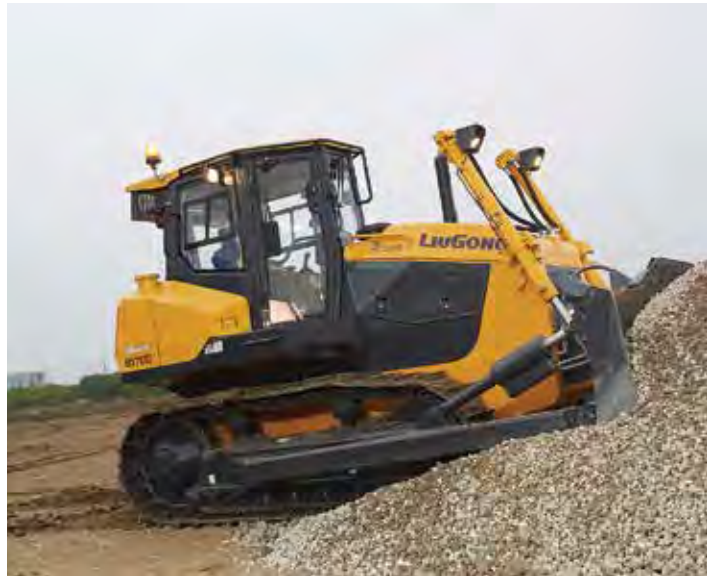
ABOVE AND BOTTOM: The new LiuGong B170D bulldozer is available in two types, Standard and Wetland, with an operating weight of 17,500 kg/19,500 kg and a blade capacity of 4.5 cu m.
