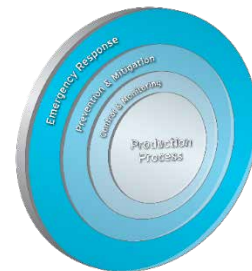
Figure 2: Both the safety standard and the cyber security standard prescribe separate protection levels. Image courtesy of HIMA Paul Hildebrandt GmbH
