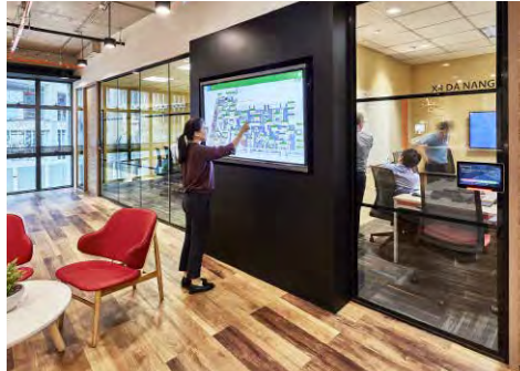
A digital dashboard shows at a glance which rooms are being occupied, temperature at various parts of the office and energy usage in real-time. Photo: © Sodexo
